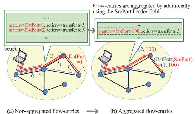
Figure 2. Flow aggregation of the flow-entries.
