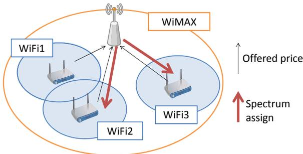
Figure 3: Channel assignment
