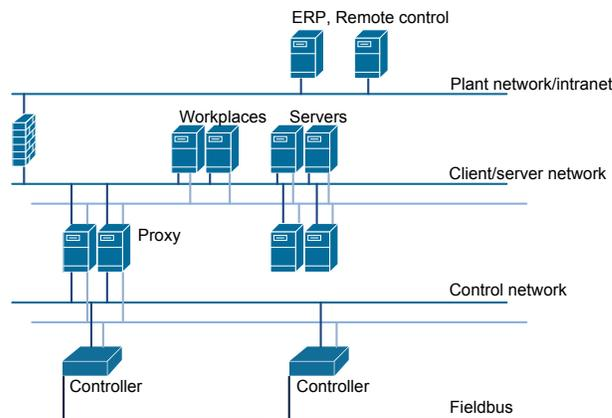
Fig. 1. An example of automation network architecture
