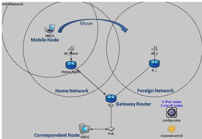
Figure 1: Simulation environment for MIPv6 and MCoA scenarios
