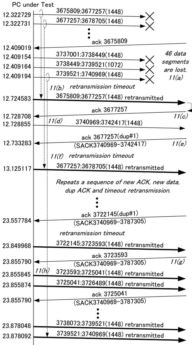
Figure 11. Timeline of segment exchanges at OS X (2)
