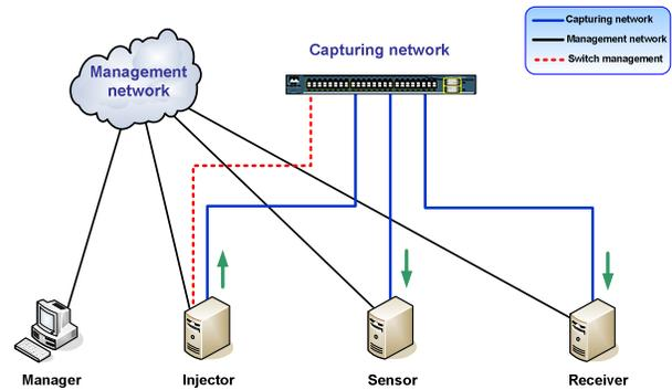
Figure 5. Network infrastructure to test the probes.
