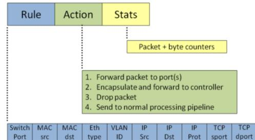
Figure 2. The OpenFlow Flow Entry [11]
