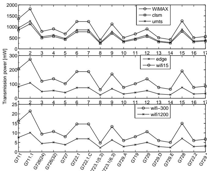
Figure 9: Transmission power consumption.
