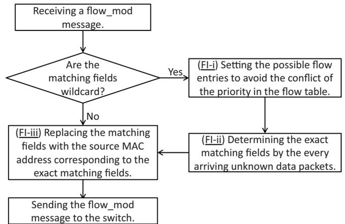
Figure 6. Summarized process of flow entry installation.
