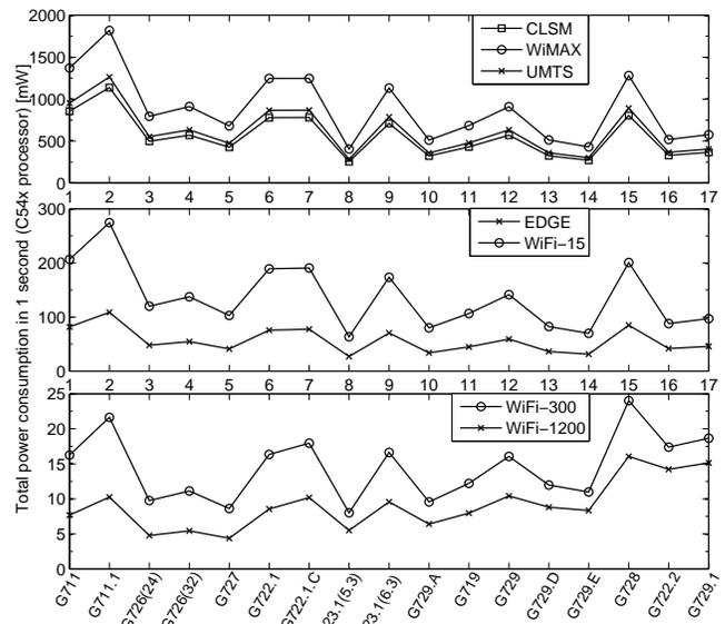
Figure 10: Total power consumption for C54x.
