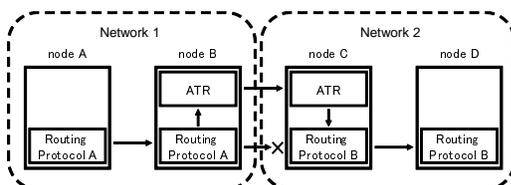
Figure 1: Behavior of ATR in heterogeneous MANET environment.
