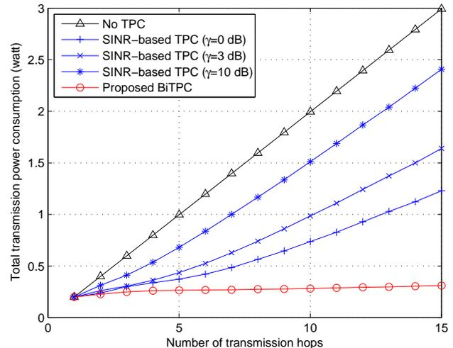
Figure 6. Total transmission power vs. number of hops.
