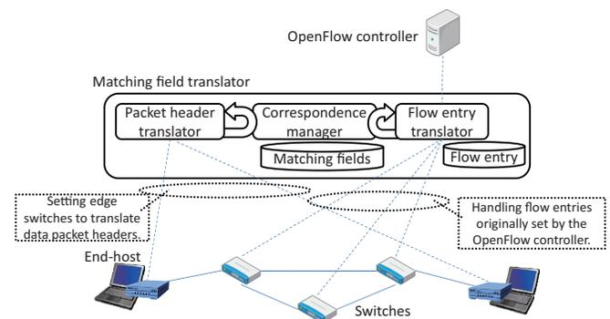
Figure 4. The architecture of the matching field translator.
