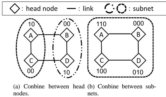
Figure 3: Group ID assignment procedure.
