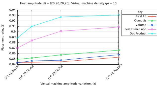
Figure 2. Increasing virtual machine amplitude variation non-uniformly.
