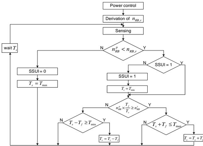
Figure 5. Flow chart of proposed sensing algorithm.
