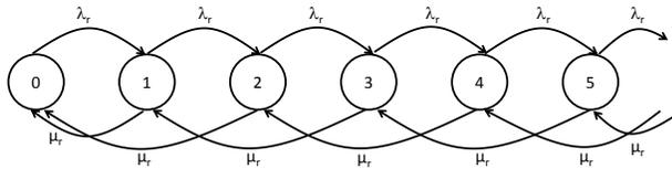
Figure 4. State transition diagram of the relay's queue.
