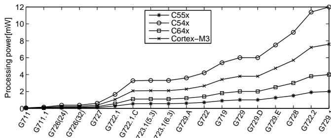
Figure 5: Encoding power consumption of voice codecs.
