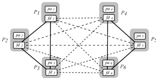
Fig. 1: Application topology with failure detector  $\mathcal{P}$
