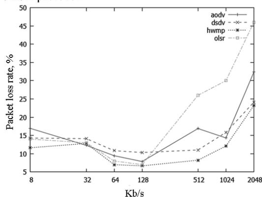
Figure 4. Packet loss rate from data transmission rate.
