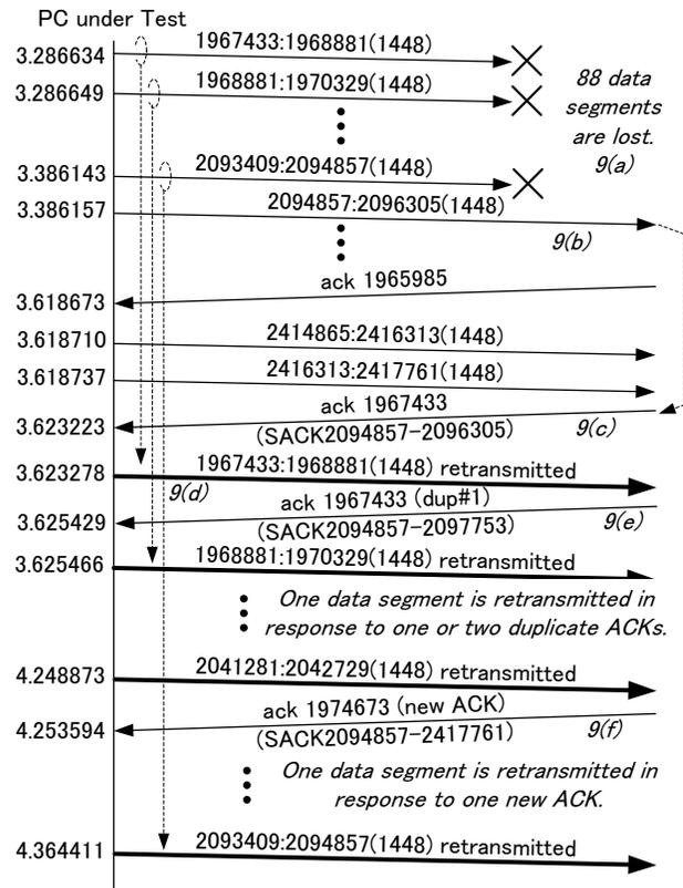
Figure 9. Timeline of segment exchanges at Reno (1)
