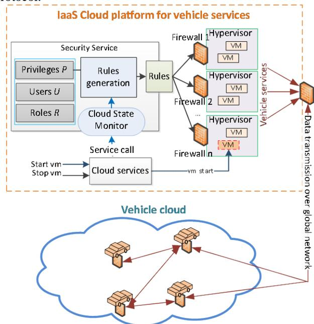
Figure 7. Security platform for cloud oriented ITS.
