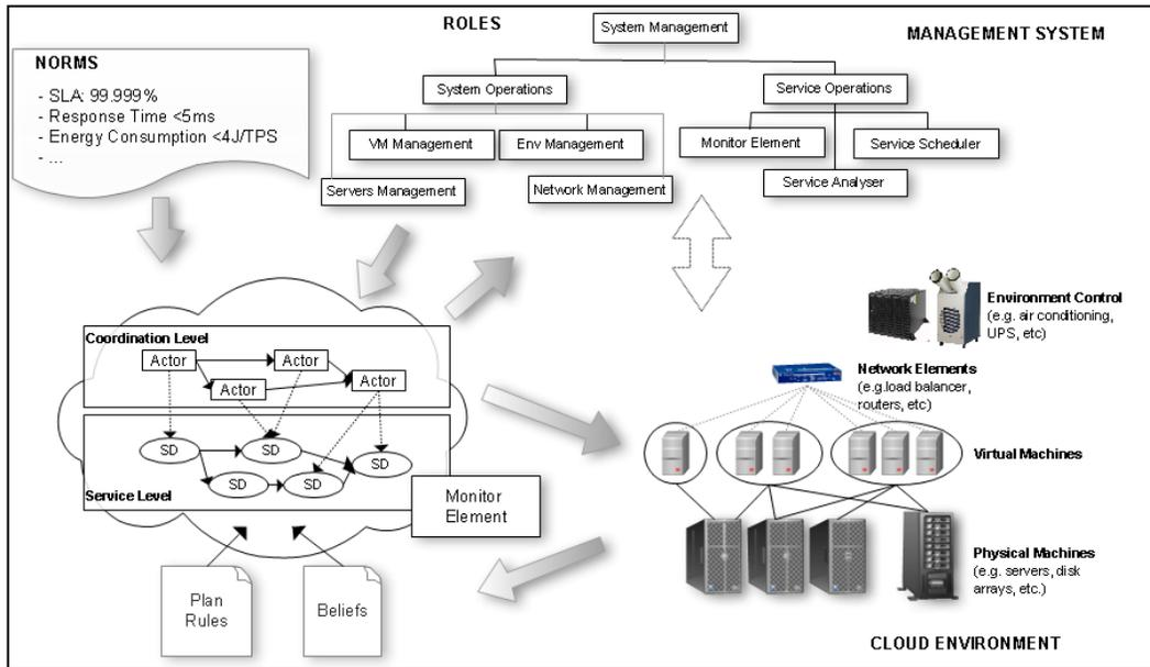
Figure 2 – Green Cloud management system based on OTM [6].
