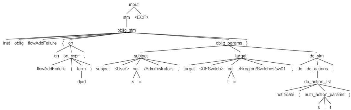
Figure 5. The AST tree for Listing 9 example
