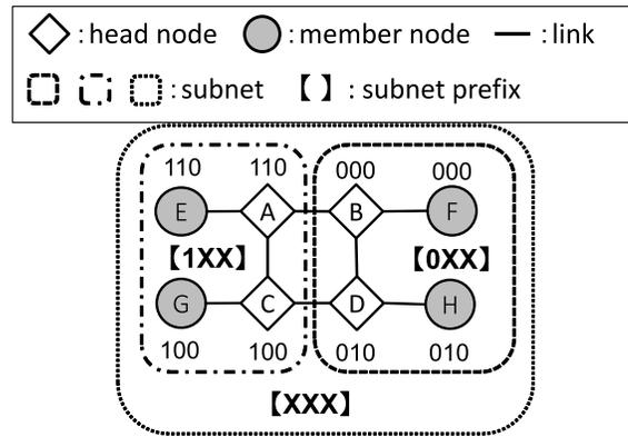
Figure 4: Result of group ID assignment procedure.
