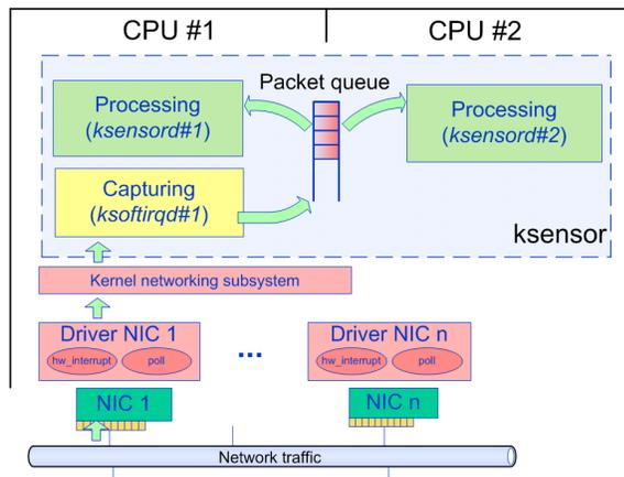
Figure 4. Execution instances in Ksensor with two processors and one NIC.
