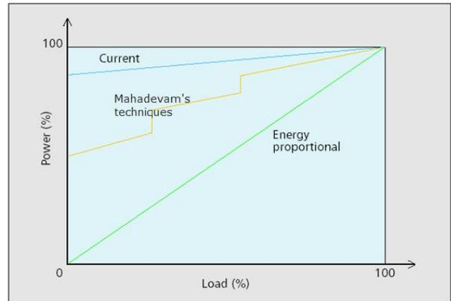
Figure 1 - Consumption in computer networks as a function of the workload [5].
