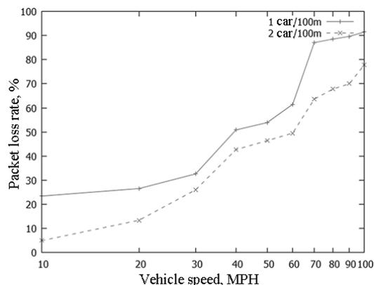
Figure 5. Packet loss rate from vehicle speed
