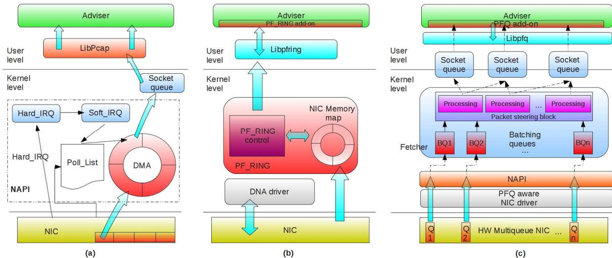
Figure 2. Adviser capturing packets (a) with NAPI and LibPcap (b) with PF\_RING (c) with PFQ.
