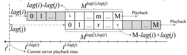
Figure 1. Buffers states mapping with playback lags
