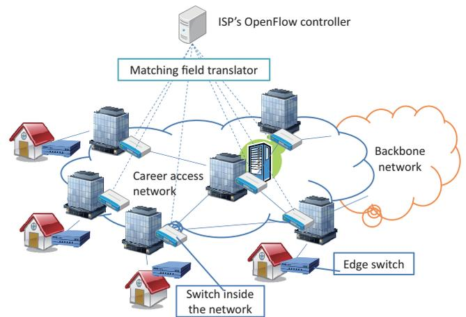
Figure 5. Deployment in a carrier access network.
