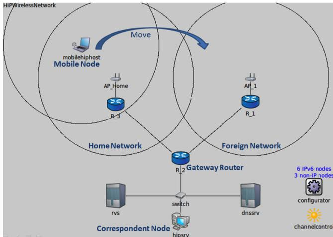
Figure 2: Simulation environment for HIP scenarios
