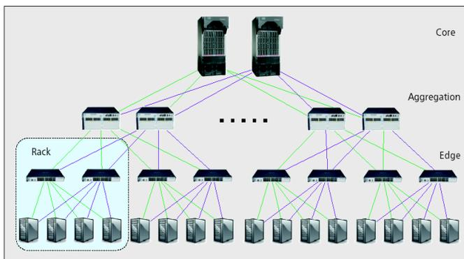
Figure 3- Typical network topology of a datacenter [5].
