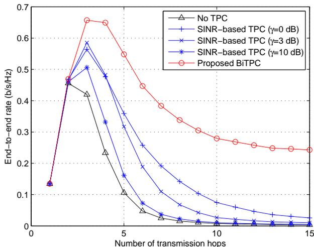
Figure 5. End-to-end rate vs. number of hops.
