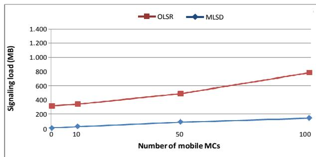
Figure 4. Signaling overhead
