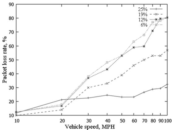
Figure 6. Packet loss rate while transmitting emergency message.
