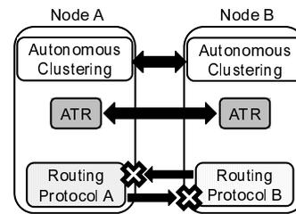
Figure 2: Protocol design of the proposed inter-domain routing.
