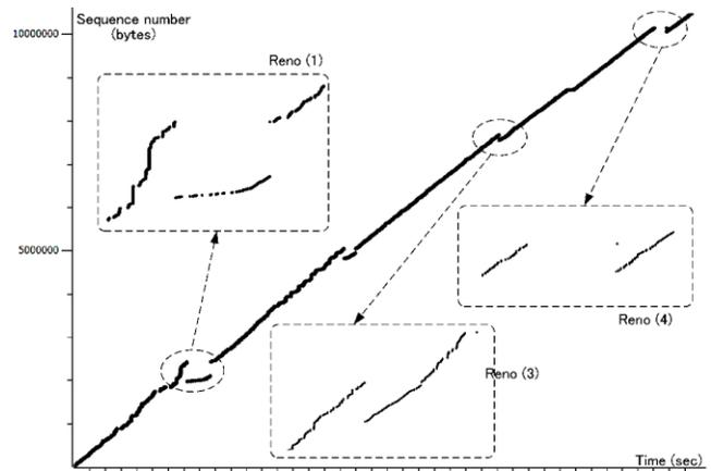
Figure 2. Sequence number vs. time for TCP Reno
