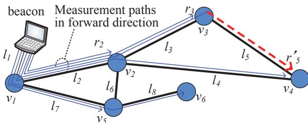
Figure 1. The calculation of the measurement paths.
