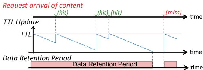
Figure 1: Traditional TTL-based caching
