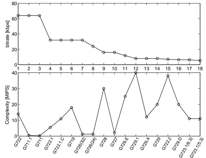
Figure 4: Complexity and bitrate for different audio codecs.
