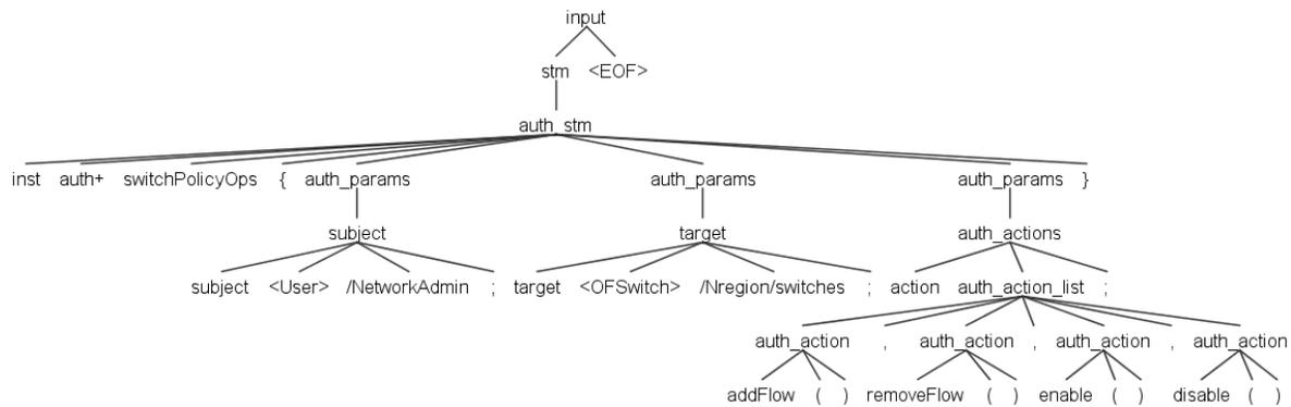
Figure 4. The AST tree for Listing 2 example
