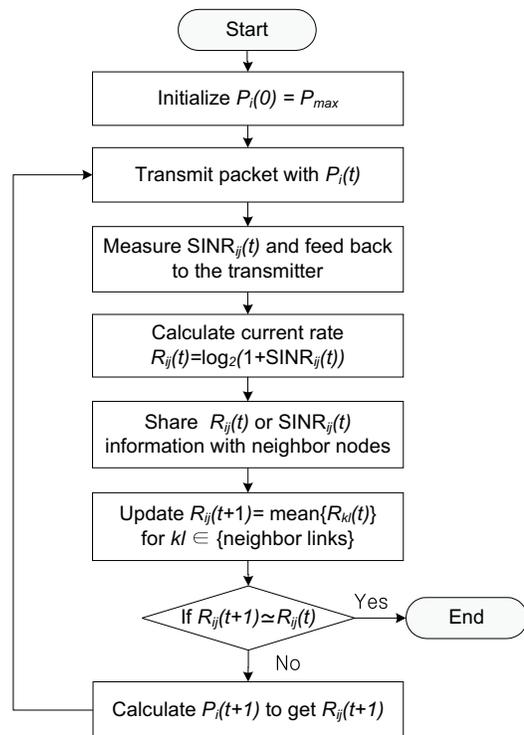
Figure 2. Flow chart of proposed BiTPC algorithm.
