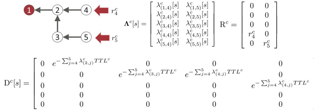
Figure 4: An example of matrices  $\Lambda^c$ ,  $\mathbf{R}^c$ , and  $D^c$  for the request propagation on the delivery tree having origin 1
