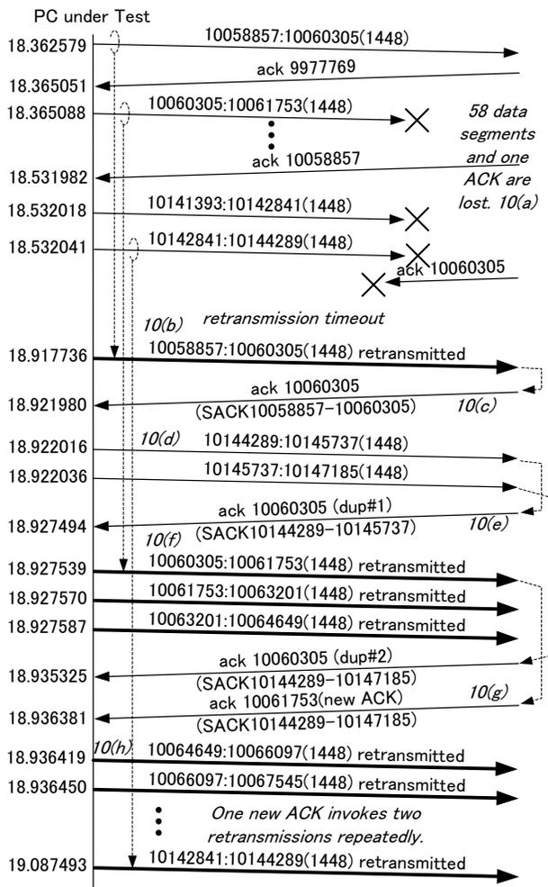
Figure 10. Timeline of segment exchanges at Reno (4)
