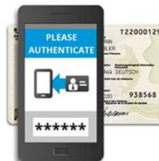
Step (1): The App asks you to hold your identity card behind the back of your smartphone and to enter the 6-digit PIN of your German eID card. [Figure 3a]
