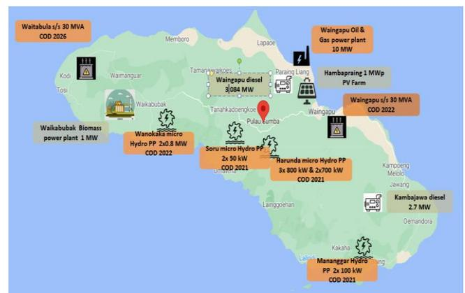
Figure 1. Sumba distribution grid and its planning expansion
