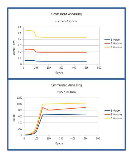
Figure 3. Simulated annealing case. Influence of the number of epochs in the obtained energy amdon the execution time
