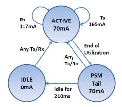
Figure 3. Typical power state machine of a Wi-Fi antenna [19]
