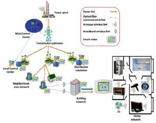
Figure 1. Hierarchical communication networks in a SG model [16]
