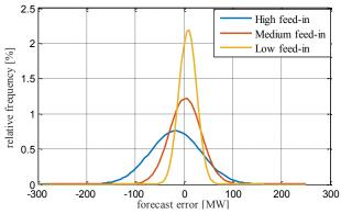
Figure 2. Normal distribution of Forecast Errors over a year of different feed-in levels.
