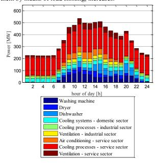
Figure 4. Profile of Available Load Shifting Power
