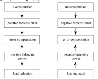
Figure 3. Connection between the type of forecast error and suitable countermeasures.
