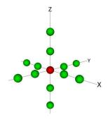
Figure 3. Seismic wave propagation stencil [9].
