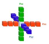
Figure 4. Acoustic wave propagation stencil [10].
