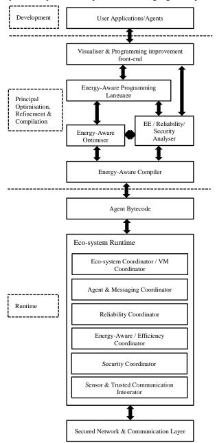
Figure 1. PLECO Eco-system architecture
