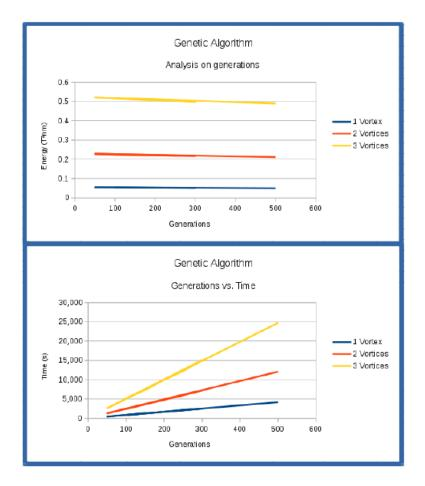
Figure 2. Genetic algorithm version of the code. Influence of the generations on the energy obtained and the executiont time
