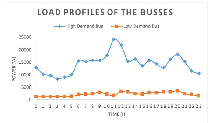
Figure 5. Load curves of the high/low demand busses connected to the adjustable transformer in Saarland (Germany).
