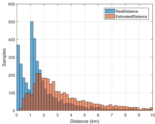
Figure 6. Comparison between estimated and real fault distances.
