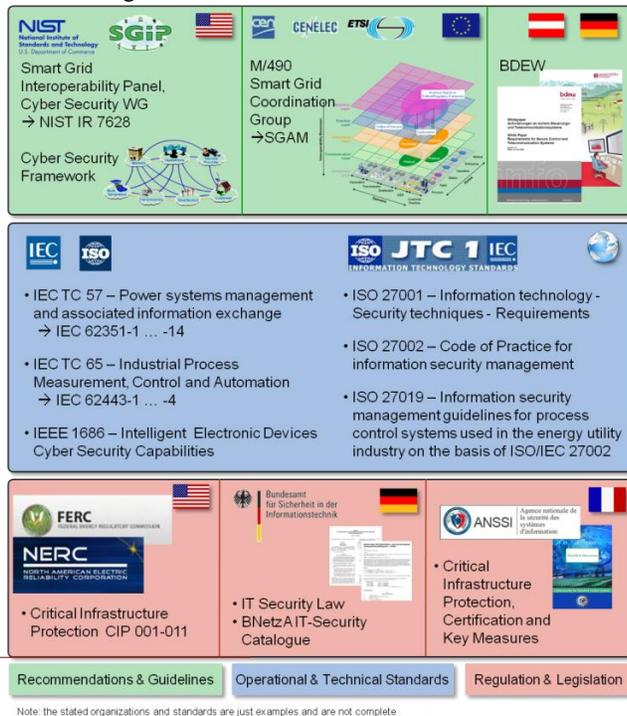
Figure 2. Examples for sources for security requirements for digital grid
