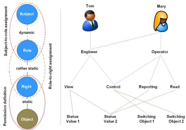
Figure 4. Basic RBAC concept applied in Digital Grids
