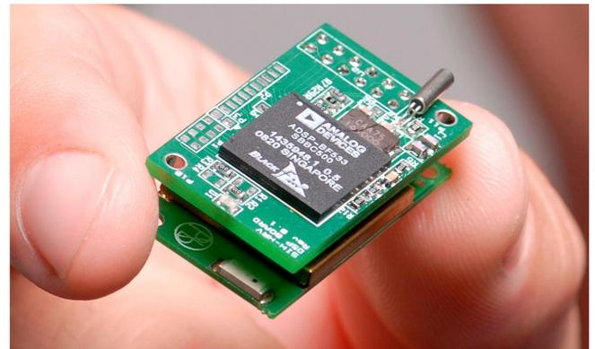
Figure 4. The physical ASE-BAN gateway module. The size is 13 mm x 18 mm x 30 mm. The weight is approximately 6 g.
