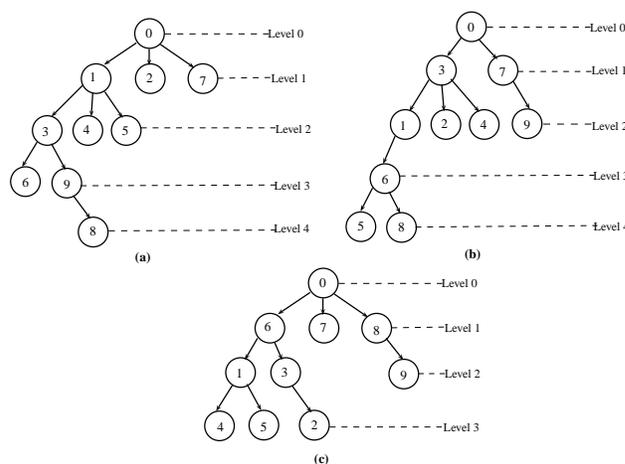
Figure 5: (a) Tree obtained with WASP-No LPL (b) Tree obtained with WASP-LPL-100ms (c) Tree obtained with WASP-LPL-150ms
