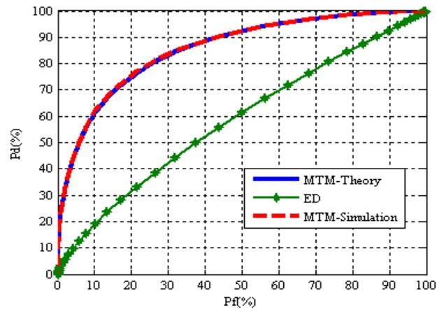
Fig. 1. Probability of detection versus probability of false alarm using MTM with  $NW=4$  and 5 tapers (simulation and theory) and the periodogram (energy detector) at AWGN with  $SNR=-10dB$  and  $L = 20$ .
