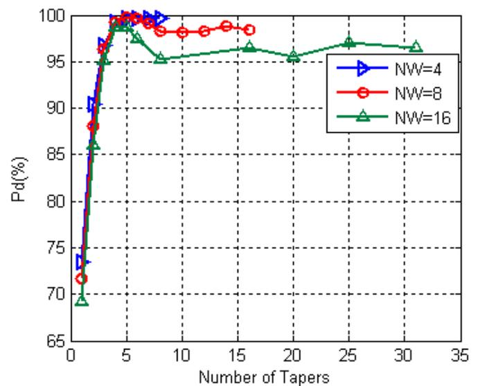
Fig. 5. Probability of detection versus number of tapers ( $K$ ) using MTM with different half time bandwidth products ( $NW$ ) where the probability of false alarm was 10% and at channel AWGN with  $SNR = -5$ dB.
