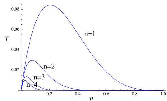
Fig. 6: Channel achievable transmission rate  $T$  in bits/s/Hz as a function of the hop distance (expressed in number of intermediary nodes  $n$ ).  $\theta = 10\text{dB}$ ,  $\sigma = 4\text{dB}$ , links SINR=10dB.
