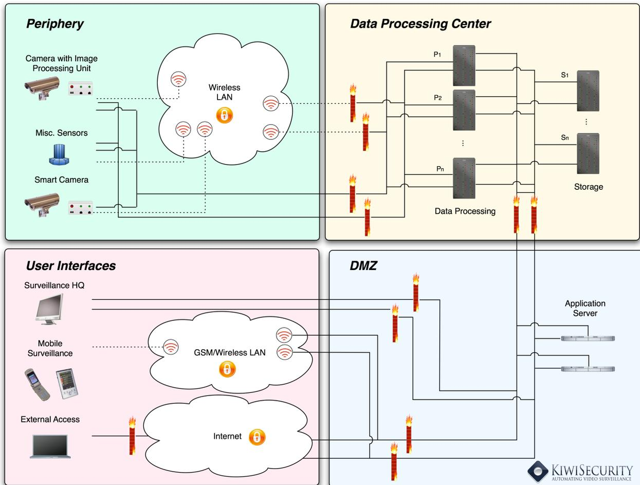
Figure 2: System architecture of the NIVSS system
