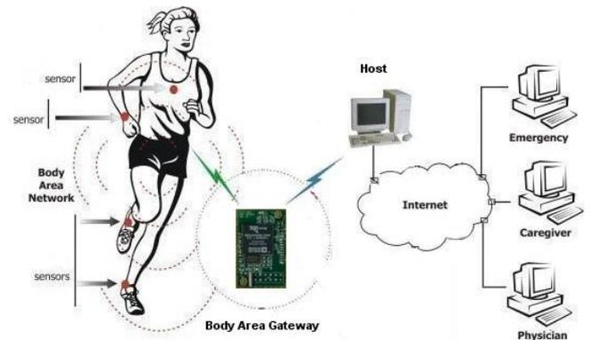
Figure 1. The wireless body area network.
