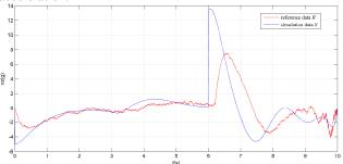
Figure 2. Comparison between reference and simulation lateral acceleration
