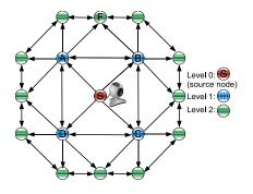
Figure 4. P2P topology. S is the source peer.
