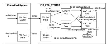
Figure 4. Data Flow for the Filtering Process
