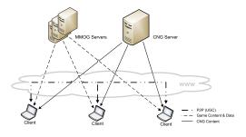
Figure 1. CNG architecture.
