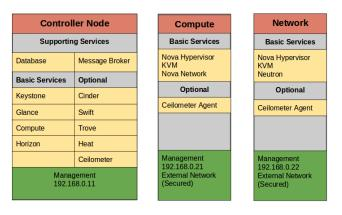
Figure. 2. Architecture of Openstack based Cloud.
