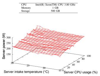
Figure 3. A typical server power model constructed by the neural network method
