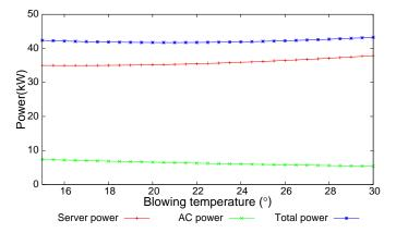
Figure 10. Power consumption of servers, power consumption of air conditioner, and total power consumption of data center versus air-conditioner blowing temperature
