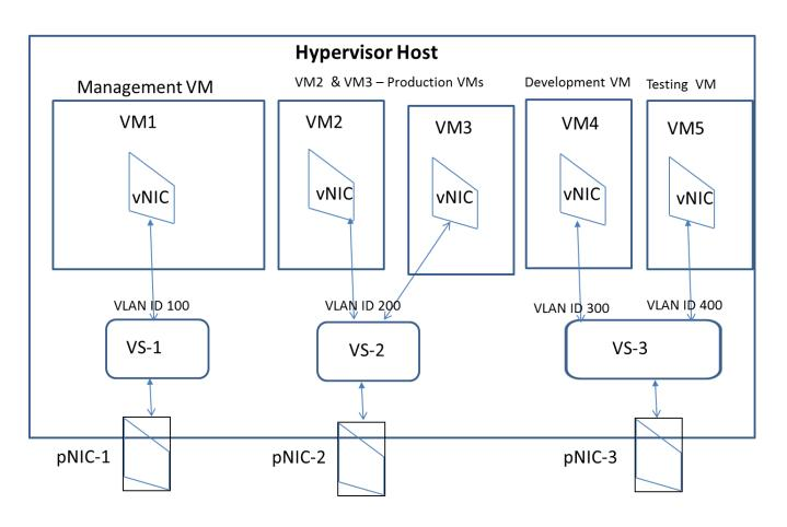
Figure 1 - VLAN-based Network Segmentation
