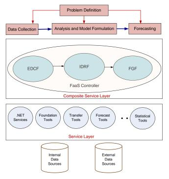
Figure 1. A SOA-based framework for the forecasting process
