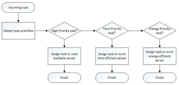
Figure 1. Flow chart of proposed algorithm functionality
