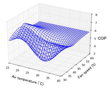
Figure 4. Air-conditioner power model constructed by support vector regression method
