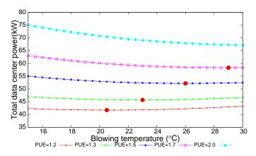
Figure 13. Total power of the data center and the air temperature that minimizes the power consumption of the data center for PUE values of 1.2, 1.3, 1.5, 1.7, and 2.0
