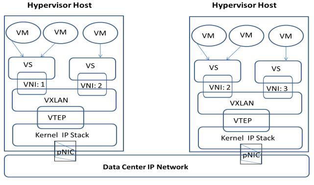
Figure 2 - Overlay-based Virtual Network Segmentation
