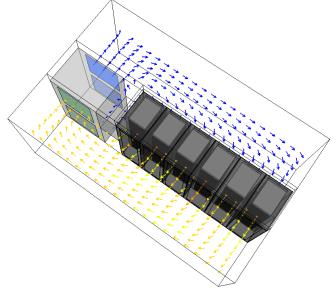
(b) Conventional arrangement with cold aisle and hot aisle
