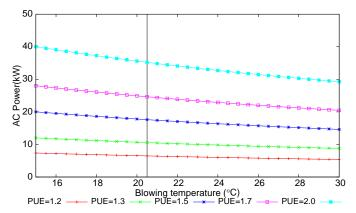
Figure 12. Power consumption of the air conditioner for PUE values of 1.2, 1.3, 1.5, 1.7, and 2.0
