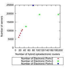
Figure 7. Number of hybrid optoelectronic routers vs number of accommodated servers (12 optical ports).
