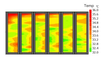
Figure 9. Air temperature distribution of the data center after VM reallocation (RMSE: 0.23)
