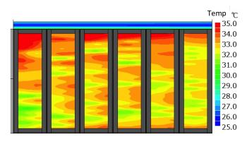
Figure 5. Temperature distribution in the exhaust-side plane of the rack when VMs are assigned to servers randomly
