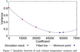
Figure 7. Quadratic function of rack exhaust temperature variances and coefficient
