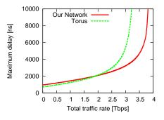
Figure 4. Comparison of the maximum delay among the server rack pairs.
