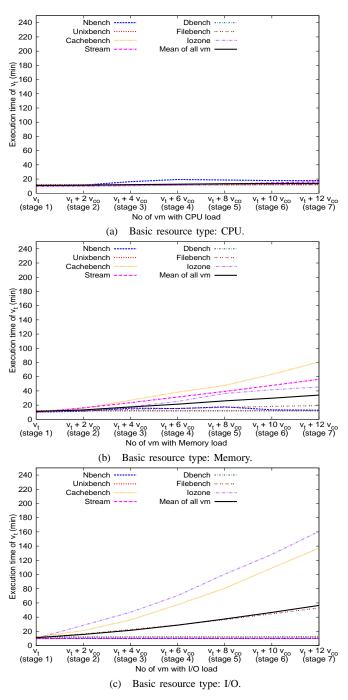
Figure 3. The TETV of  $v_t$  due to various basic types of resource load on  $v_{co}$ .
