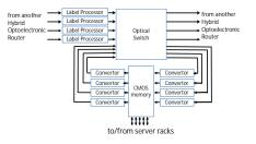
Figure 1. Hybrid optoelectronic router.
