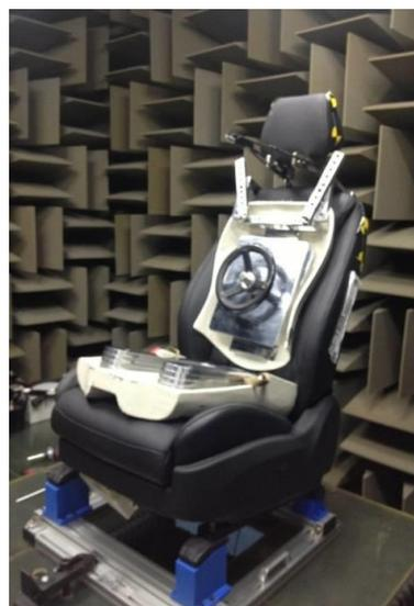
Figure 9. Experimental setup for the performance test of seat motion by applying the proposed control method in the dead sound chamber.
