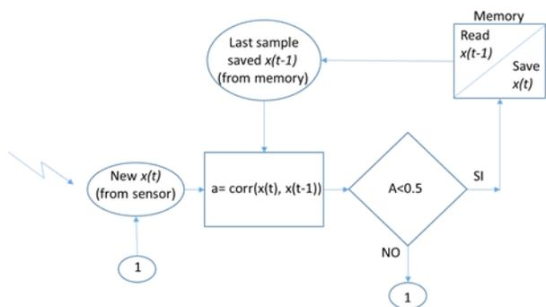
Figure 3. Monitoring process algorithm
