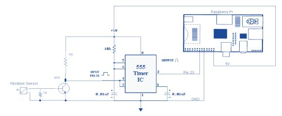
Figure 5. Schematic of Vibration Sensor Circuit.
