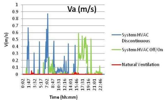
Figure 12. Typical air velocity
