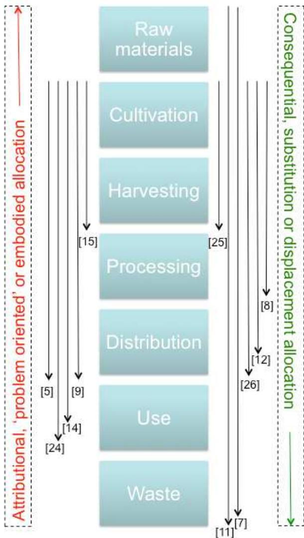
Figure 1. Examples of contrasting system boundary definitions in microalgae biofuel LCAs and related system studies (ref. Table 1)
