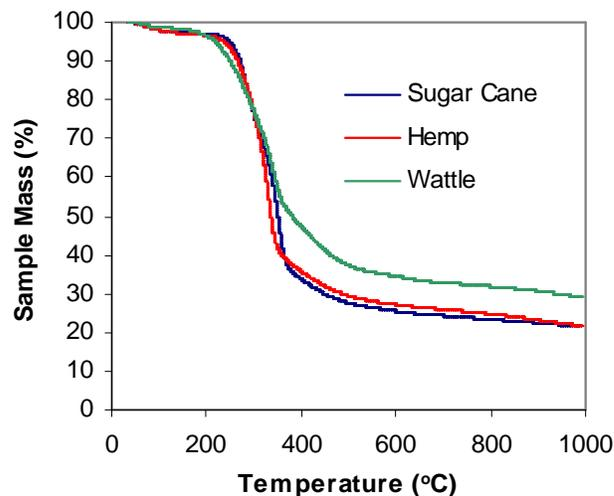
Figure 3. Thermogravimetric analysis of the biomass samples.
