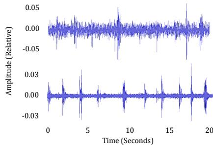
Fig. 4. Post-processing of the audio signal corresponding with water can dramatically improve signal-to-noise ratio. The top shows the original waveform. The bottom shows the waveform after a bandpass filter is applied.
