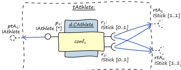
Figure 17. Allocation of component interfaces to template interfaces.
