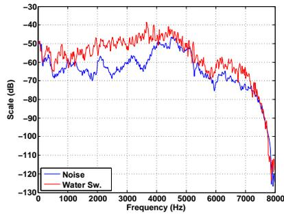
Fig. 3. Frequency distribution of a water swallow vs. silence (noise). This graph reveals that the frequency range between 500 Hz and 1000 Hz is the point of interest.
