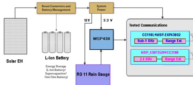
Figure 2. Implemented sensor node configurations
