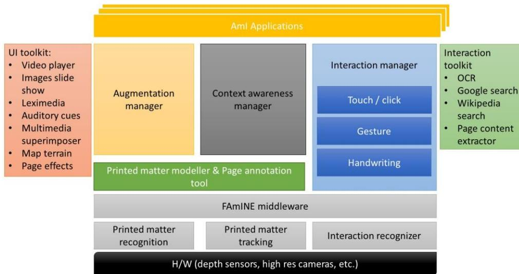
Figure 1. Framework’s architecture
