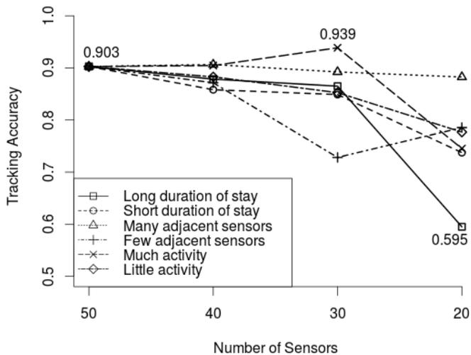
Figure 4. Tracking performance across sensor subsets by size.
