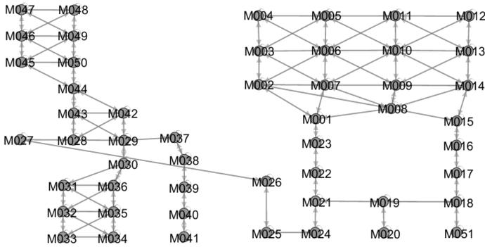
Figure 1. Graph of sensors (with their internal IDs and their spatial relations used in the evaluation (adapted from [17]).
