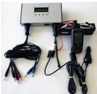
Figure 9. Electrical conductivity measurement system.
