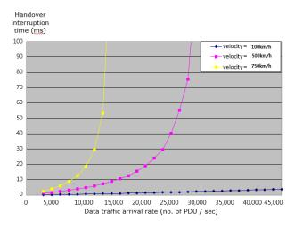
Figure 6. Handover interruption time according to traffic arrival rate.
