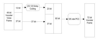
Figure 3. Hybrid FEC encoder block diagram for vocoder in [8].
