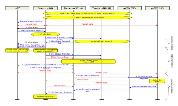
Figure 4. Handover procedure using window between mVE and mNBs.
