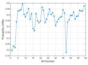
Figure 5. Bit probabilities in vocoder voice frame (calculated using 100 hours, over 19 million voice frames of AMBE 3600 bps record).
