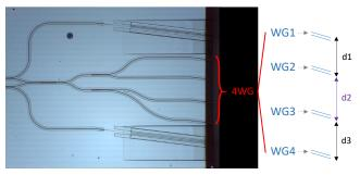
Figure 2. Measurements of the distance between the 4 waveguides (WG) at the end of the 3 asymmetric coupler network.
