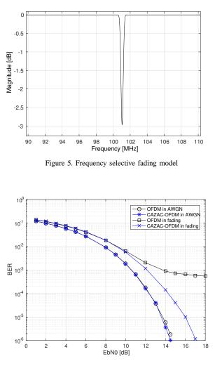
Figure 6. BER versus EbN0 under AWGN and frequency selective fading environments
