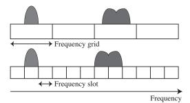
Figure 1. Frequency grids and slots.
