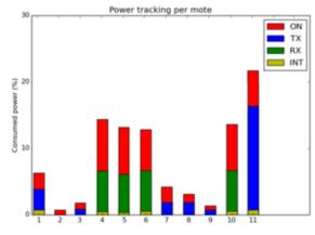
Figure 8. The Consumed Power with Flooding attack.
