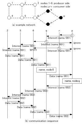
Figure 3. Communication sequence between consumer and producer.
