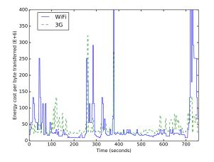
Figure 4. Energy cost per transferred byte for each network interface for a 12-minute long segment of a download process.
