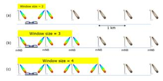
Figure 3. Assigned cases for window size. (a) Velocity is 100 km/hour as shown in subway. (b) Velocity is about 500 km/hour as shown in HST. (c) Velocity is about 750 km/hour for future HST.
