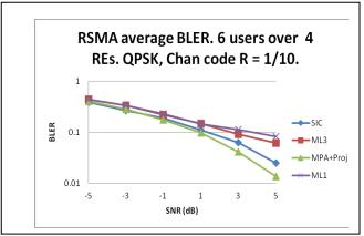
Figure 4. Simulation results for 6 users over 4REs. QPSK, Code Rate = 1/10.
