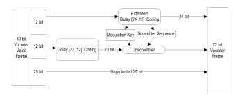
Figure 1. 3600 bps AMBE's vocoder FEC encoder scheme
