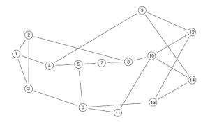
Figure 3. The 14-node network topology (NSFNET).
