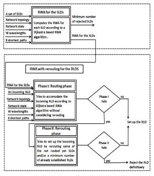
Figure 1. Block diagram of the SepRwLR algorithm.
