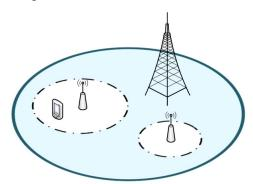
Figure 1. Representation of cellular and Wi-Fi network integration: full line circle – coverage area of a cellular network cell; dashed line circles – coverage areas of the Wi-Fi hot spots.
