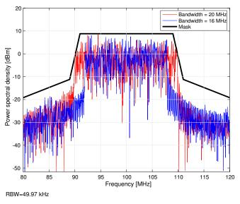
Figure 8. Spectrum for proposed system
