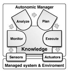
Figure 1. Mape-K Autonomic Control Loop [14].
