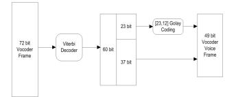
Figure 4. Hybrid FEC decoder block diagram for vocoder in [8].
