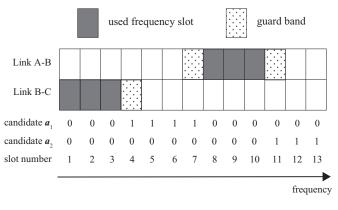
Figure 3. An example of spectrum allocations.
