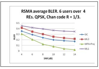
Figure 3. Simulation results for 6 users over 4REs. QPSK, Code Rate = 1/3.
