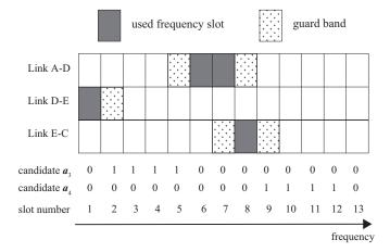
Figure 5. Path  $p_2$  and its candidate spectrum allocations.
