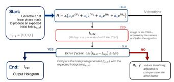
Figure 4. Block diagram of the algorithm applied for the optimization of the CGH.
