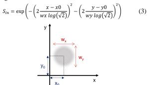
Figure 3. Diagram in Cartesian coordinate system describing the parameters (x0, y0) and (wx, wy) used for the estimation of the Input beam  $S_{in}$ .
