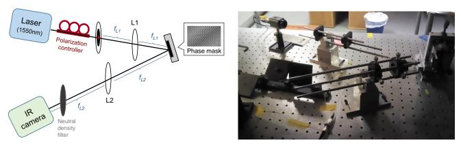
Figure 6. Left figure: Scheme of the hologram reconstruction system, using a laser of 1550nm, a polarization controller, lens L1, a LCoS-SLM, lens L2 and a IR camera. Right figure: Photography of the setup presented in the left figure.
