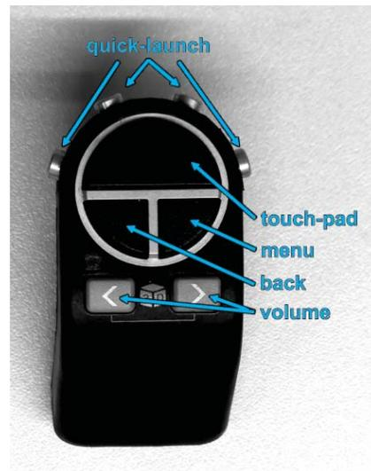
Figure 3. The Reticle Speed Mouse, a finger-worn input-device, with its standard button assignment. The size of the device is about 82 mm \* 27 mm \* 36 mm and can be put on one finger with the ring-strap on the backside of the device.
