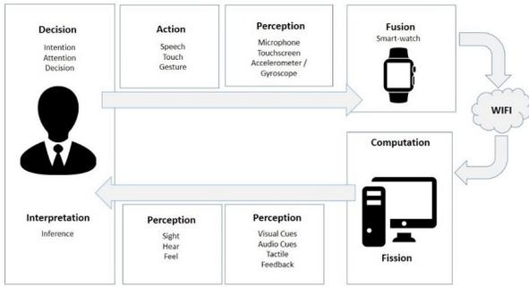
Figure 1. Multi-modal interaction system. The main components are a smartwatch and a large display enabling speech, touch, and gesture modalities perceived by the system through microphone, touchscreen, accelerometer, and gyroscope. Visual and audio cues, as well as tactile feedback are perceived by the user due sight, hear, and feel.
