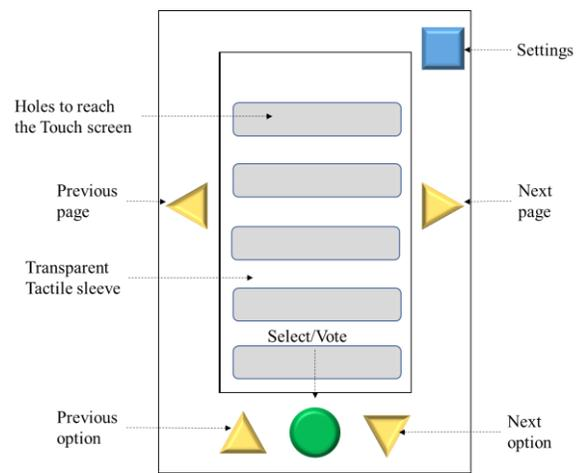
Figure 3. Voting interface with the tactile sleeve
