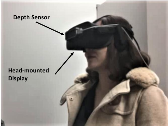
Figure 7. The remote user's wearable device: a head-mounted display with a depth sensor attached to its front side
