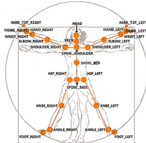
Figure 4. The 25 Joints tracked by the Kinect sensor
