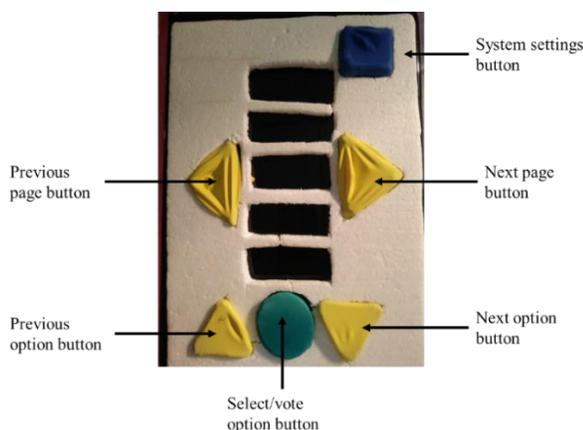
Figure 4. The prototype of the voting interface
