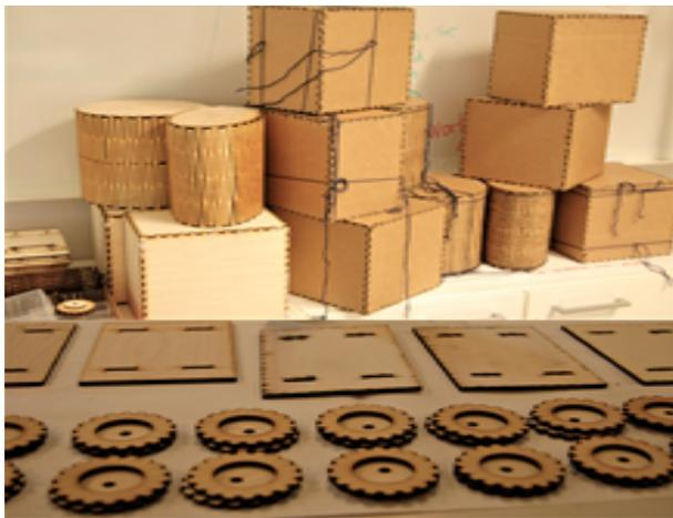
Figure 2. Top: Basic shapes. Bottom: Laser cut wheels
