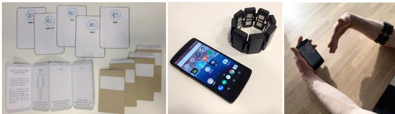
Figure 1. The mobile hand gesture toolkit including (a) Paper tools: invitation and gesture cards, (b) Hardware tools: Myo Gesture Control Armband and LG Nexus 5 phone, (c) Participant performing *Wave In* gesture
