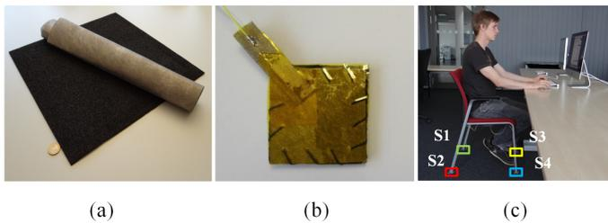
Fig. 1. System Design; a) raw materials for the pressure sensor; b) a sensor prototype; c) a chair equipped with sensors
