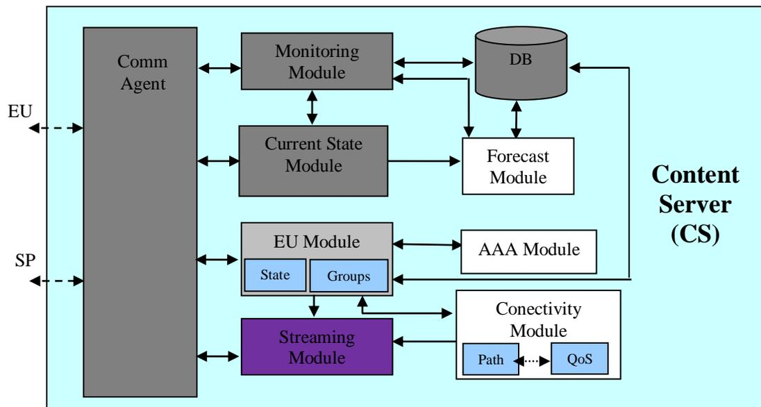
Figure 4. The Content Server software architecture
