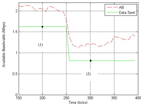
Figure 4.a Available bandwidth versus time – BART Tool scenario
