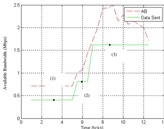
Figure 5.a Available bandwidth versus time – Pathchirp tool scenario
