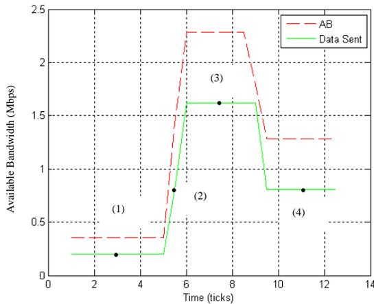
Figure 6.a Available bandwidth versus time – Passive tool scenario
