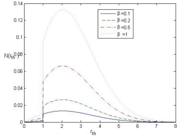
Figure 7. The level crossing rate  $N(r_{th})$  for  $r_T = 1$ ,  $\sigma = 2$ ,  $A = 0.5$  and  $\beta = 0.1; 0.2; 0.5; 1$
