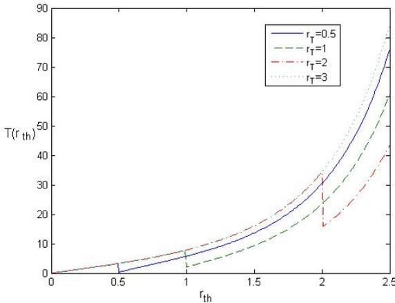
Figure 10. The fade duration  $T(r_{th})$  for  $r_T = 0.5; 1; 2; 3, \sigma = 1, A = 0.5$  and  $\beta = 0.2$
