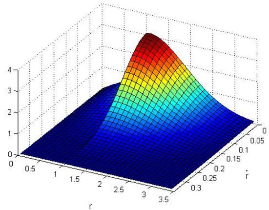
Figure 3. The joint PDF of the SSC combiner output signal and its derivative for  $r_T = 1, \sigma = 1, A = 0.5$  and  $\beta = 0.1$
