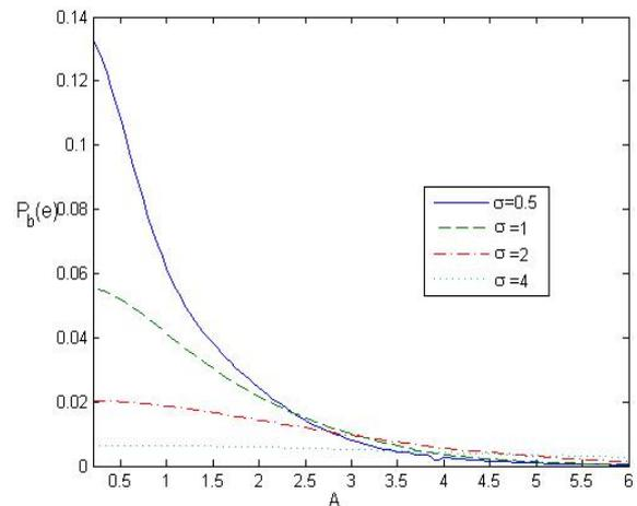
Figure 17. The bit error rate  $P_b(e)$  versus signal amplitude  $A$  for  $r_T=1, \sigma=0.5; 1; 2; 4$
