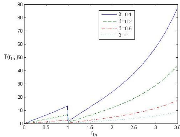
Figure 13. The fade duration  $T(r_{th})$  for  $r_T = 1, \sigma = 2, A = 0.5$  and  $\beta = 0.1; 0.2; 0.5; 1$
