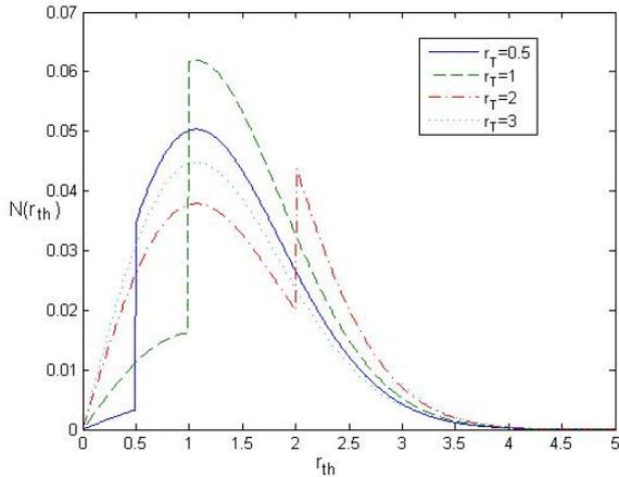
Figure 4. The level crossing rate  $N(r_{th})$  for  $r_T = 0.5; 1; 2; 3$ ,  $\sigma = 1$ ,  $A = 0.5$  and  $\beta = 0.2$
