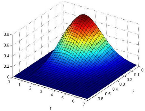
Figure 2. The joint PDF of the SSC combiner output signal and its derivative for  $r_T = 1, \sigma = 2, A = 0.5$  and  $\beta = 0.2$
