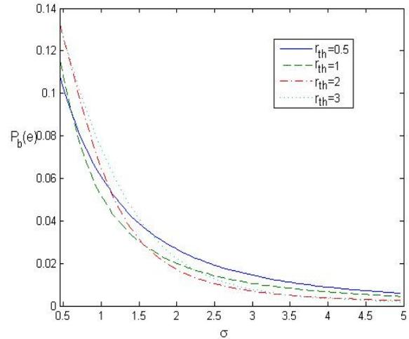
Figure 16. The bit error rate  $P_b(e)$  versus variance  $\sigma$  for  $r_T=0.5; 1; 2; 3, A=0.5$
