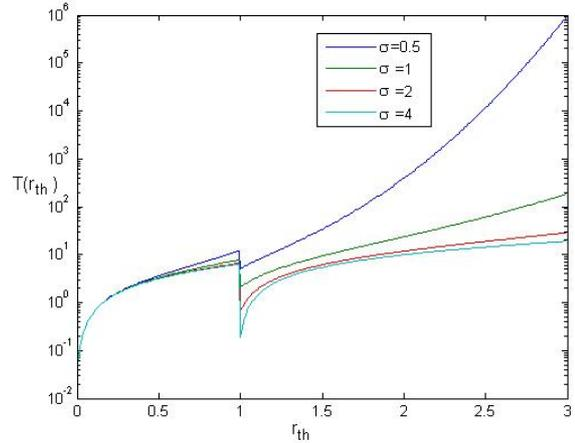
Figure 11. The fade duration  $T(r_{th})$  for  $r_T = 1, \sigma = 0.5; 1; 2; 4, A = 0.5$  and  $\beta = 0.2$
