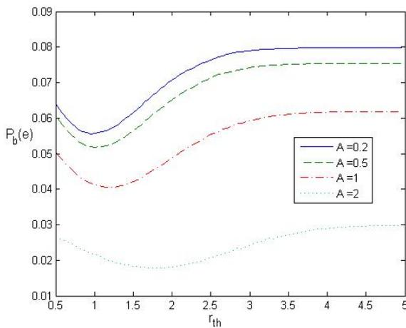
Figure 15. The bit error rate  $P_b(e)$  versus the threshold for  $\sigma=1, A=0.2; 0.5; 1; 2$
