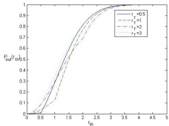
Figure 8. The outage probability  $P_{OUT}(r_{th})$  for  $r_T = 0.5; 1; 2; 3$ ,  $\sigma = 1$ ,  $A = 0.5$
