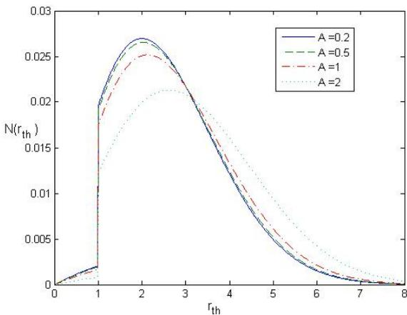
Figure 6. The level crossing rate  $N(r_{th})$  for  $r_T = 1$ ,  $\sigma = 2$ ,  $A = 0.2; 0.5; 1; 2$  and  $\beta = 0.2$
