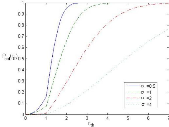
Figure 9. The outage probability  $P_{OUT}(r_{th})$  for  $r_T = 1, \sigma = 0.5; 1; 2; 4, A = 0.5$
