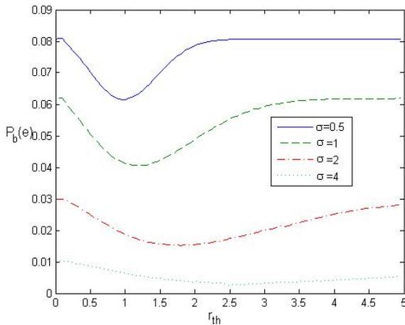
Figure 14. The bit error rate  $P_b(e)$  versus the threshold for  $\sigma=0.5; 1; 2; 4, A=1$
