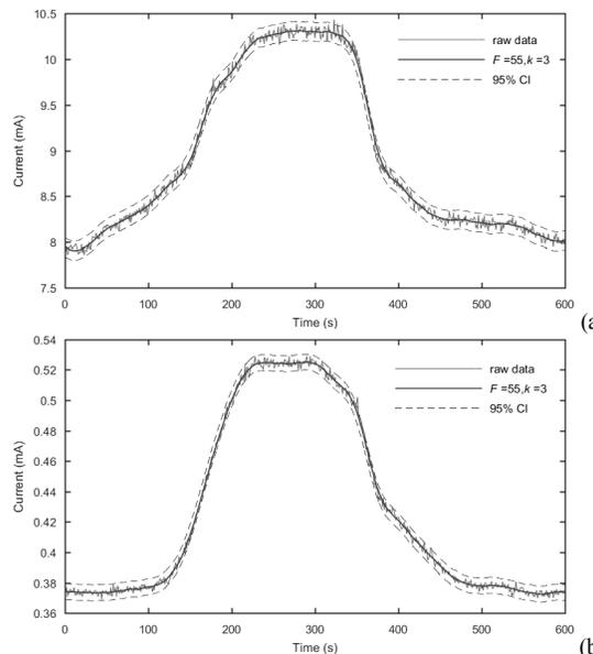
Figure 14. Plot of raw signal vs. SG smoothed signals ( $k = 3, F = 55$ ) with pointwise 95% confidence bands: (a) SZ device, (b) S1Z3 device.
