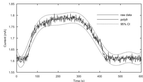
Figure 5. 9<sup>th</sup> degree fitted polynomial for the S sensor response signal.
