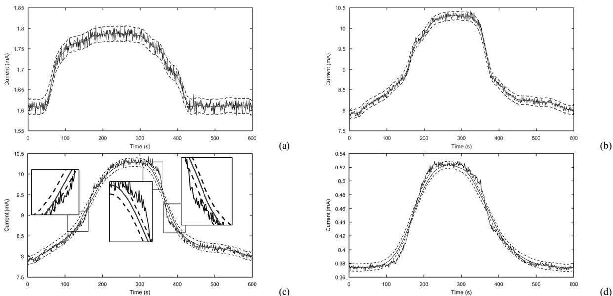
Figure 8. Raw vs smoothed signal using a MA filter: (a) S device with a span of 25, (b) SZ device with a span of 25, (c) SZ device with a span of 75 (insets) highlight some of the areas where the model is outside of the 95% confidence bands, and (d) SZZ1 device with a span of 55.
