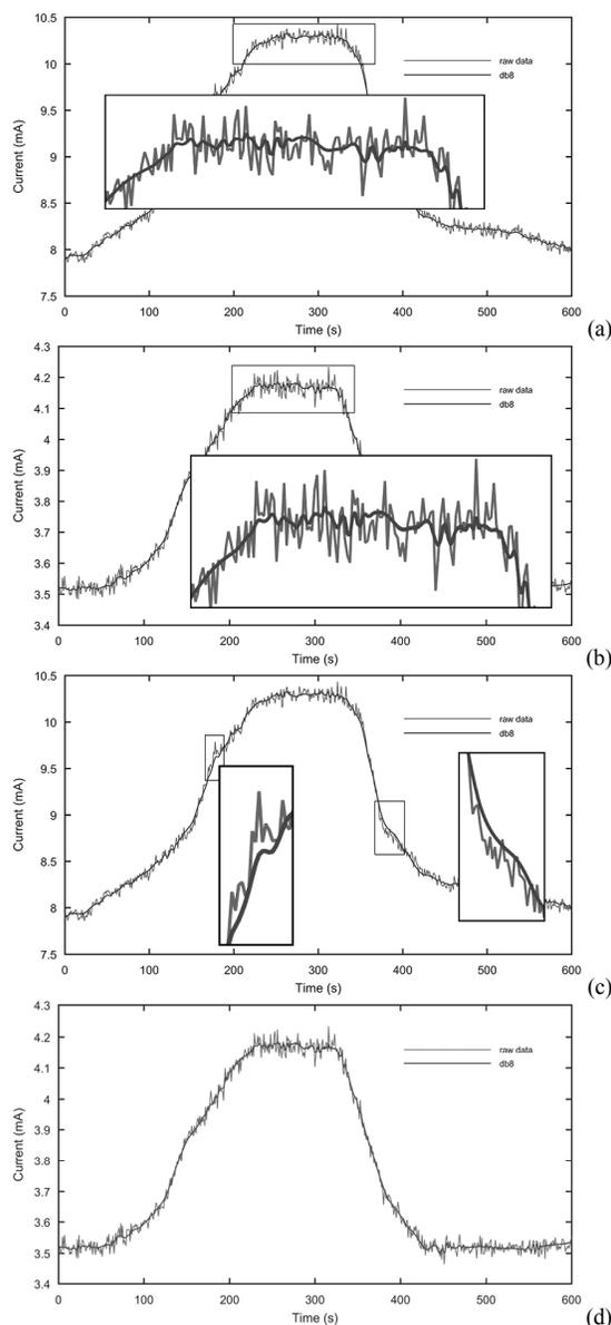
Figure 20. Plot of db8 wavelet denoised signals with original response signal for: (a)  $SZ$  sensor and (b)  $S_3Z_1$  sensor (insets show perturbations), (c)  $SZ$  sensor (insets highlight regions where the profile of the original curve is not maintained) and (d) the full  $S_3Z_1$  signal.
