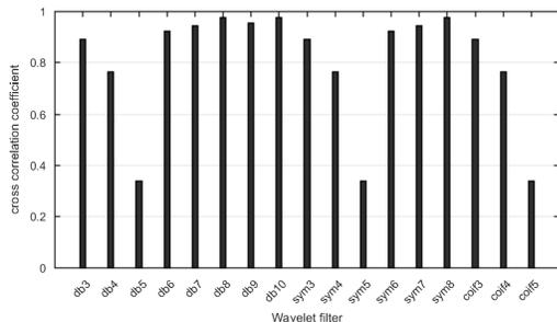
Figure 15. Comparative plot of cross correlation coefficients with selected mother wavelet filters for the S signal.
