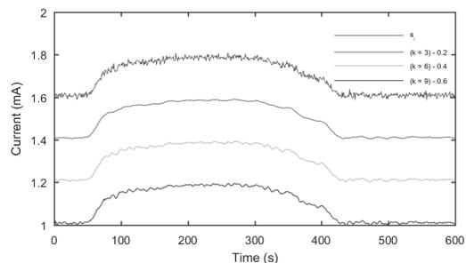
Figure 12. The effect of polynomial order on the degree of SG smoothing of the S device response signal ( $s$ ). Signals are offset for visibility.
