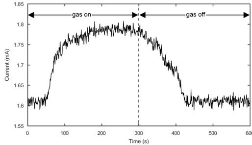
Figure 1. A typical gas sensor signal.
