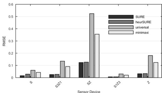
Figure 16. Comparative plot of SURE, heurSURE, universal and minimaxi thresholding schemes for all five MOX gas sensor response signals.
