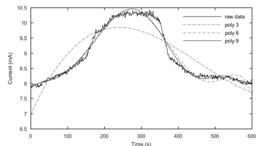
Figure 4. 3<sup>rd</sup>, 6<sup>th</sup> and 9<sup>th</sup> polynomial curve fitting for the SZ sensor response signal.
