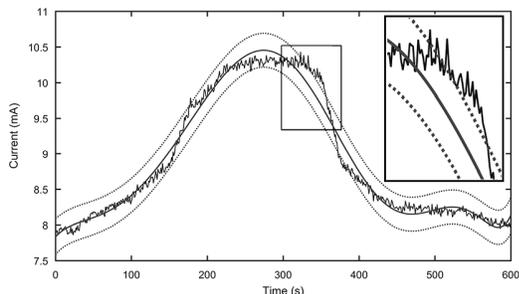
Figure 6. 9<sup>th</sup> degree fitted polynomial for the S<sub>Z</sub> sensor response signal (inset) showing data outside of the 95% CIs for the model.
