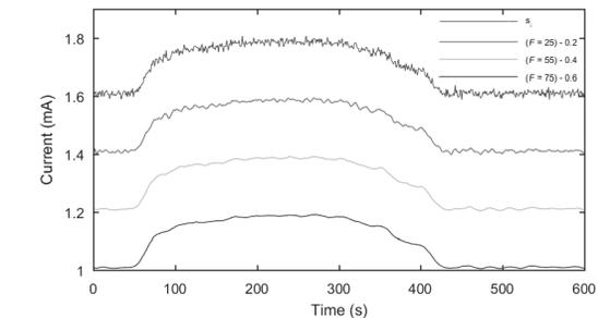
Figure 13. The effect of frame size ( $F$ ) on the level of smoothing for the S signal using a cubic polynomial. Signals are offset for visibility.
