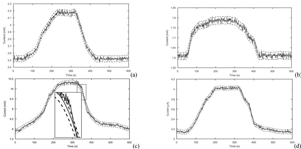
Figure 10. Smoothing with a 10% span using loess: (a) SZZ1 signal and (b) S signal and roloess curve filtering (c) SZ device signal filtering using a 20% span, (d) Z device signal filtering using a 10% span.
