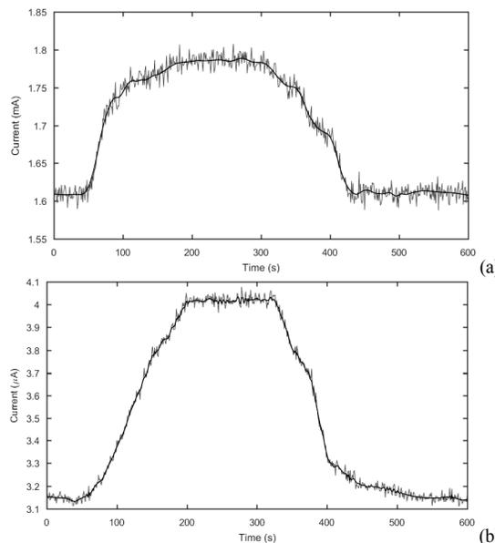
Figure 17. Plot of raw vs. wavelet denoised S (a) and Z (b) sensor signals with optimal mother wavelet (db8) and soft thresholding (with SURE).
