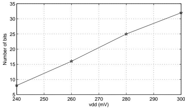
Fig. 19. Number of carry circuits or bit obtained from carry chain when supply voltage is varied.
