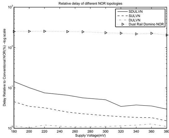
Fig. 6. Relative delay of three ULV topologies Dual Rail domino NOR to conventional NOR.
