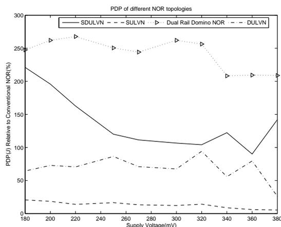
Fig. 11. Motecarlo simulation for PDP of three ULV topologies Dual Rail domino NOR relative to conventional NOR.
