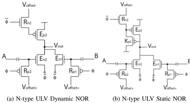
Fig. 2. NP domino dynamic and static ULV NOR gate.
