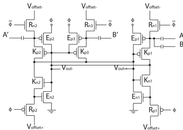
(b) Static differential P-type ULV NOR<sup>2</sup>/NAND<sup>2</sup>.
