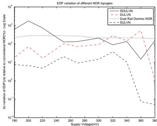
Fig. 14.  $3\sigma$  variation of EDP for SDULVN, DULVN, SULVN relative to conventional NOR.
