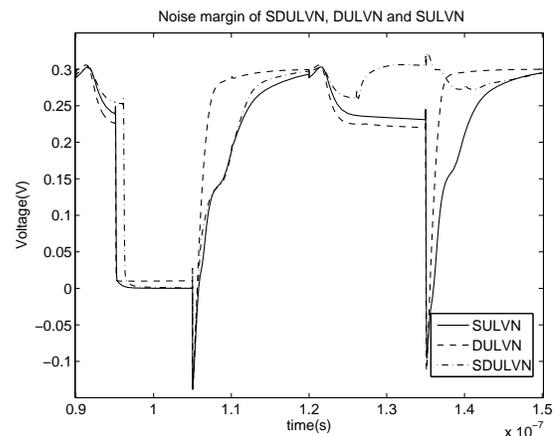
Fig. 5. Noise margin of SDULVN compared to DULVN and SULVN. Supply voltage of 300 mV.
