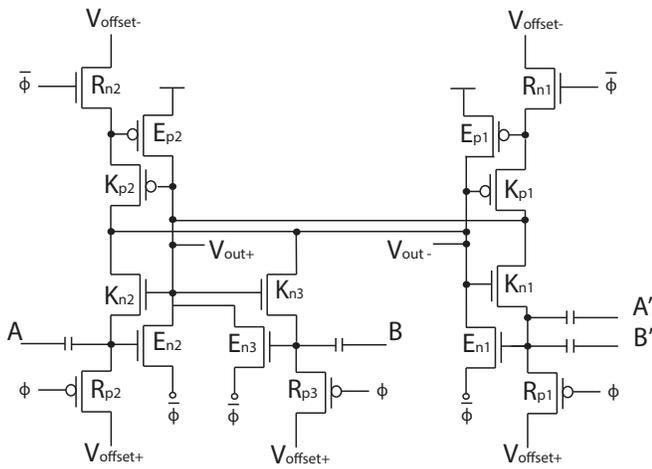
(a) Static differential N-type ULV NOR<sup>2</sup>/NAND<sup>2</sup>.
