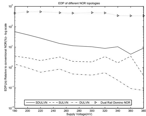
Fig. 12. Motecarlo simulation for EDP of three ULV topologies and Dual Rail domino NOR relative to conventional NOR.
