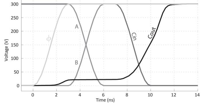
Fig. 17. Carry input and output for SULVC gate. Supply voltage at 300mV.
