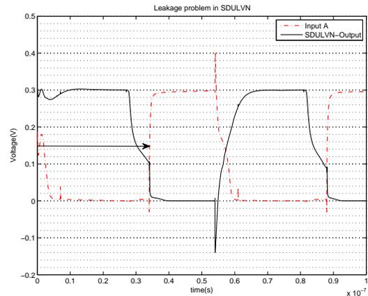
Fig. 4. Output of SDULVN where input is delayed and the output tends to shift before input due to leakage current. The graph is taken from Monte Carlo simulation in order to show why the limits for functional circuits are set as they have been discussed. Supply voltage at 300 mV.
