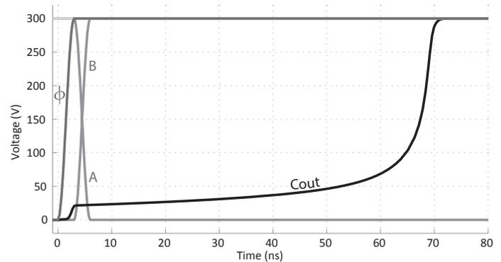
Fig. 18. Drifting problem of the SULVC output.
