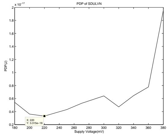
Fig. 9. PDP of SDULVN. Graph shows the Minimum Energy Point
