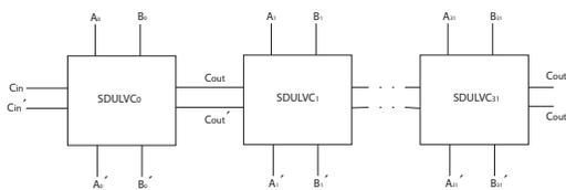
Fig. 22. 32 bit ULV carry chain.
