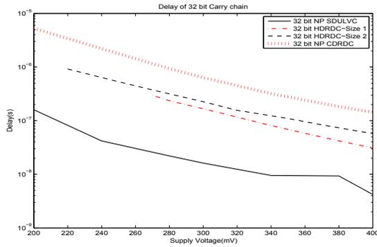
Fig. 25. Delay of 32 bit SDULVC and hybrid dual rail domino at varied supply voltage.
