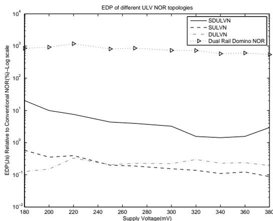
Fig. 8. Relative EDP of three ULV topologies and Dual Rail domino NOR to conventional NOR.
