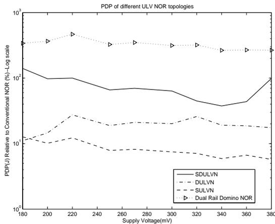
Fig. 7. Relative PDP of three ULV topologies Dual Rail domino NOR to conventional NOR.
