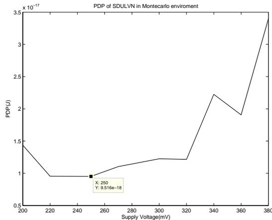
Fig. 10. PDP of SDULVN in Monte Carlo environment. Graph exhibits shift in Minimum Energy Point.
