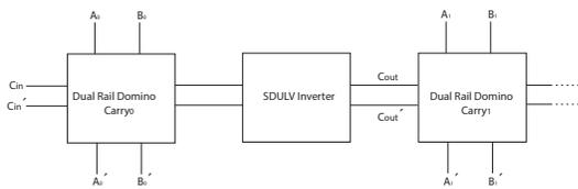
Fig. 23. Implementation of hybrid Dual rail domino carry.
