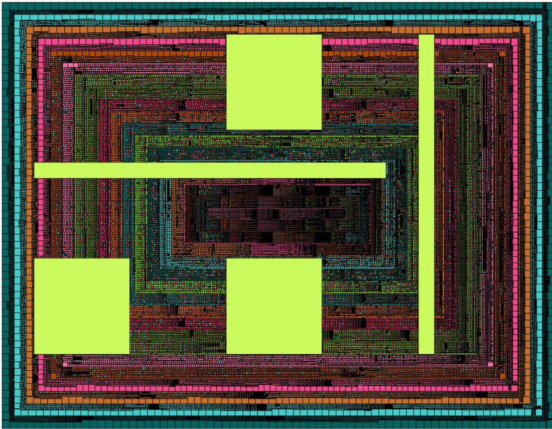
Figure 4. The packing of 97,272 randomly generated items in a rectangular surface. The application is multithreaded, each thread associated with a rectangular border. 5 large lime-green rectangles with different geometries are placed in various locations before the computation starts.
