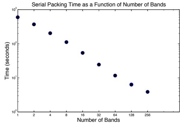
Figure 7. Running times for packing 1,000,000 rectangles with 1 to 256 bands dividing the packing area. User times measured on one core of a 3.5 GHz 64-bit AMD 8-core processor.
