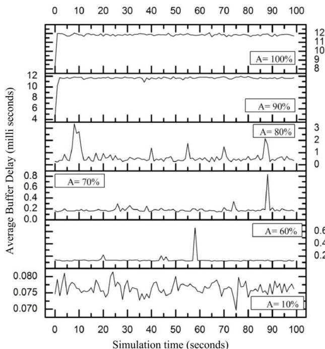
Figure 7. Average Buffer Delay for the associated passive channel of ONU<sub>0</sub> using the first case of traffic distribution (25% of A destined to Metro<sub>0</sub> and 75% of A destined to CO<sub>1</sub>). Results are presented for five values of Offered Traffic  $A = [100\%, 90\%, 80\%, 70\%, 60\%, 10\%]$ .
