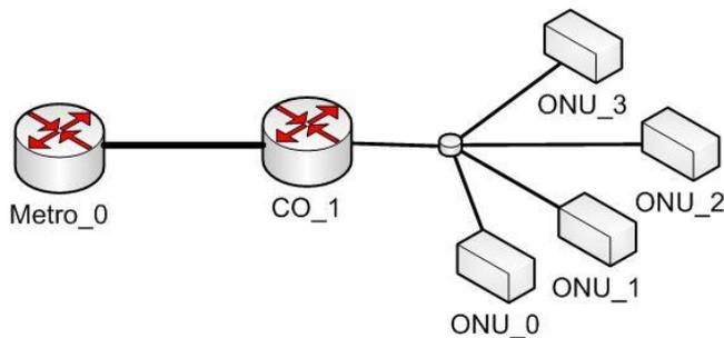
Figure 4. Validation scenario. Four Optical Network Units (ONU) connected through a Passive Optical Network to a Central Office (CO\_1), the CO\_1 is connected to the Metro-Access interfacing node (Metro\_0).
