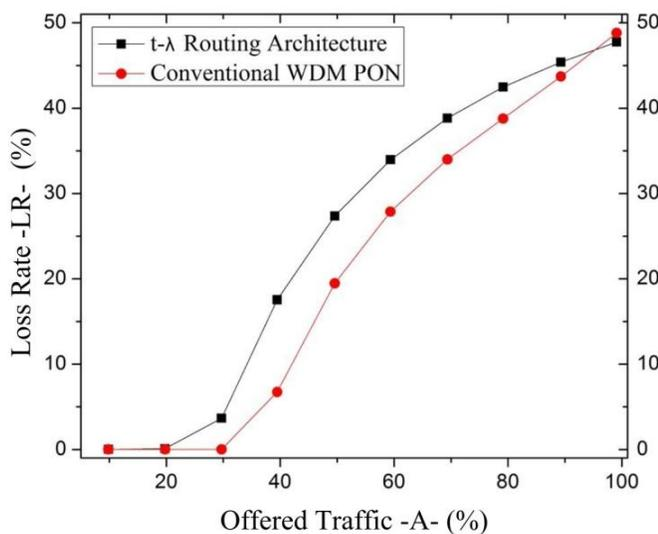
Figure 10. Loss Rate (*LR*) vs. Offered Traffic ( $A$ ); for 70% of  $A$  destined to Metro Node (MN).
