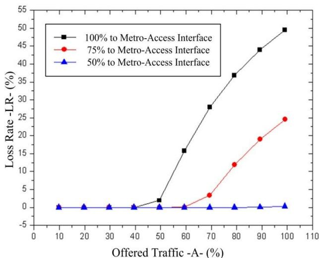
Figure 8. Loss Rate (LR) vs. Offered Traffic (A) for the WDM-PON Architecture. The three curves represents diferent traffic distributions.
