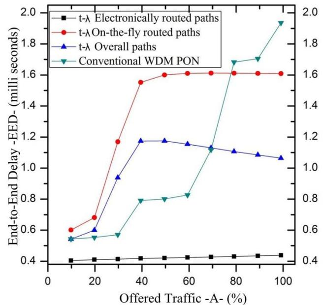
Figure 11. End-to-End Delay (*EED*) vs. Offered Traffic ( $A$ ); for 70% of  $A$  destined to Metro Node (MN).
