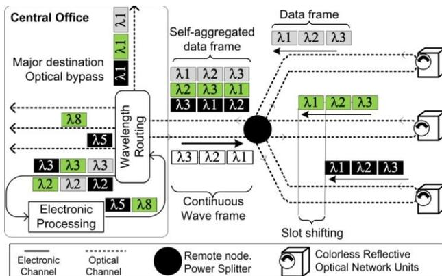
Figure 2. Underlying idea of the time-wavelength assignment and Central Office (CO) schematic diagram, for time-wavelength routed architecture to provide on-the-fly routing to Major destinations. CW: Continuous Wave.
