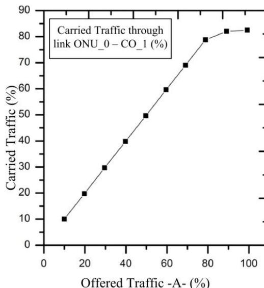
Figure 6. Carried Traffic ( $A_c$ ) vs. Offered Traffic (A) for link ONU<sub>0</sub> – CO<sub>1</sub> using the first case of traffic distribution (25% of A destined to Metro<sub>0</sub> and 75% of A destined to CO<sub>1</sub>).
