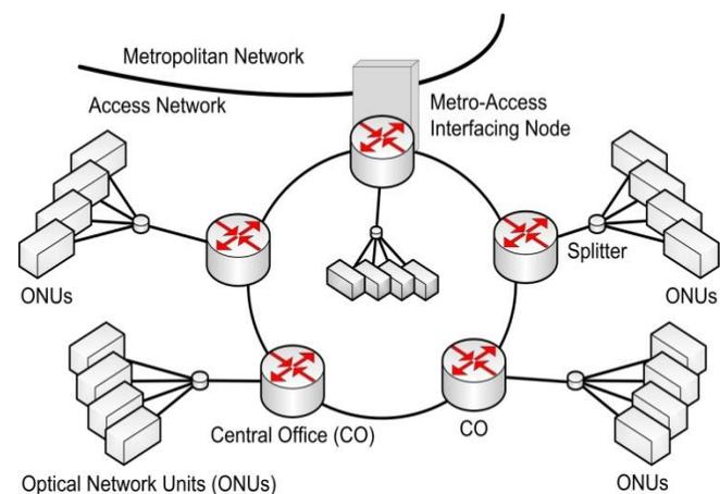
Figure 9. Simple Access network topology used for the performance evaluation, based on a ring interconnection of COs. The Metro-Access interfacing Node (MN) represents the major destination (for the performance assessment up to 70% of traffic was destined to MN).
