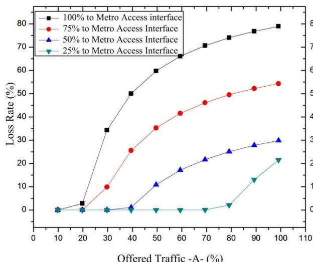
Figure 5. Loss Rate (LR) vs. Offered Traffic (A) for the  $t-\lambda$  Routing Architecture. The four curves represents diferent traffic distributions.
