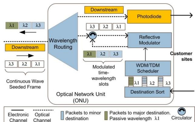
Figure 3. Basic Reflective Optical Network Unit (ONU) scheme. Downstream and Upstream channels coming from the Central Office (CO) are separated by a wavelength filter. The seeded upstream Continuous Wave (CW) is modulated and reflected back to the CO by the colorless reflective semiconductor optical amplifier (RSOA). Incoming customer traffic is sorted by destination in specific buffers.
