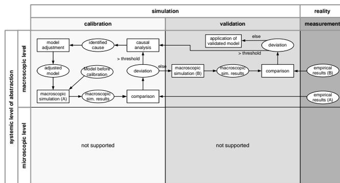
Fig. 3. Calibration and validation of a macroscopic simulation model on macroscopic level
