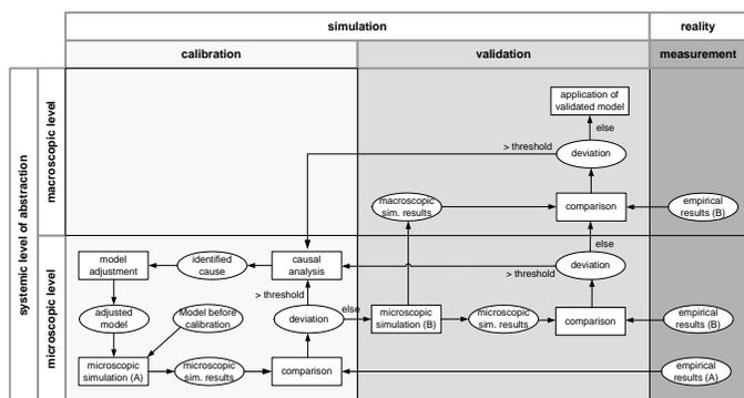
Fig. 5. Calibration and validation of a microscopic simulation model on microscopic and macroscopic level
