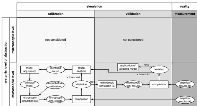
Fig. 2. Calibration and validation of a microscopic simulation model on microscopic level
