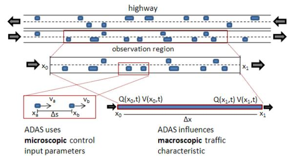
Fig. 1. Driver assistance system perception at the microscopic and macroscopic levels
