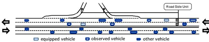
Fig. 8. Measurement concept with several cars
