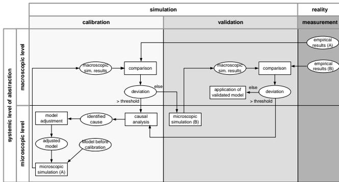
Fig. 4. Calibration and validation of a microscopic simulation model on macroscopic level
