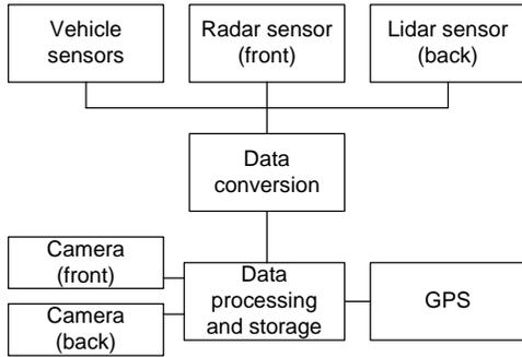
Fig. 7. General layout of the in-vehicle measurement system
