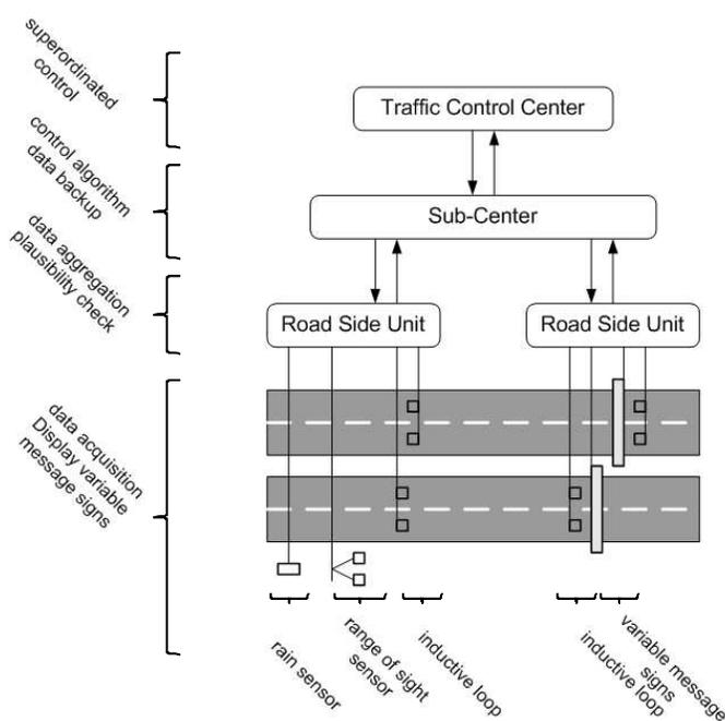
Fig. 6. System layout of a traffic control center
