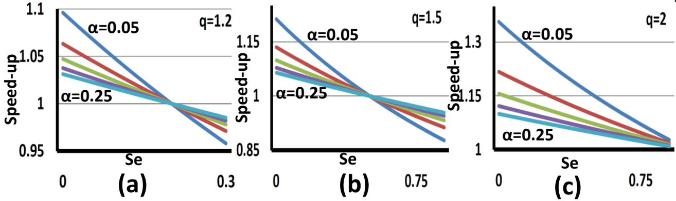
Fig. 3. Performance analysis of overclocking with error rate for different memory bounded workloads (a) Overclocking at 1.2X (b) Overclocking at 1.5X (c) Overclocking at 2X
