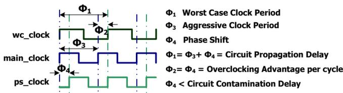
Fig. 2. Timing diagram showing overclocking advantage per cycle, as compared to the worst-case clock
