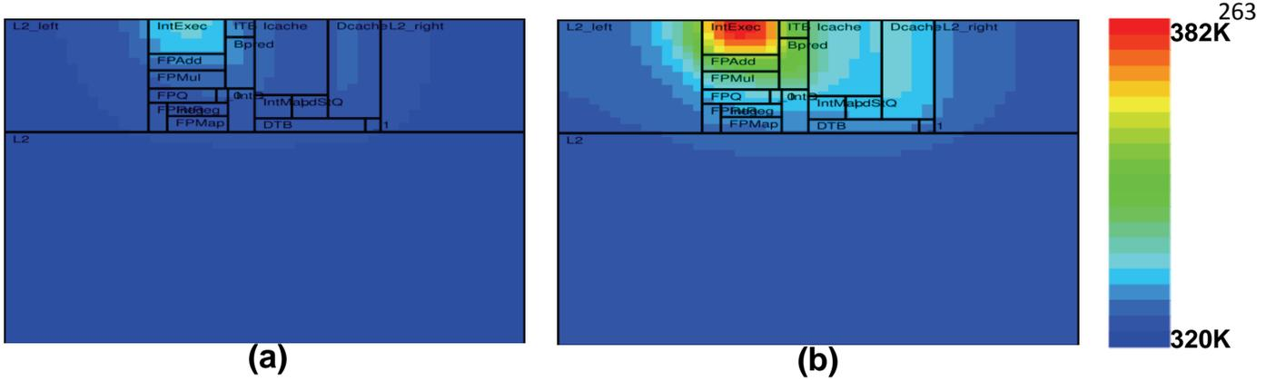
Fig. 5. Steady state temperature analysis (a) Non-overclocked processor settles around 330K (b) Reliably overclocked processor reaches over 380K
