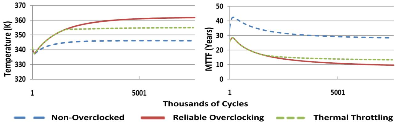
Fig. 11. *mcf* (a) On-chip Temperature Trend (b) MTTF Chart
