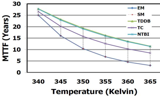
Fig. 4. MTTF for different steady state temperatures
