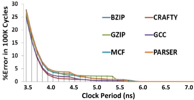
Fig. 7. Cumulative error rate at different clock periods for the IVM processor executing instructions from SPEC INT 2000 benchmarks
