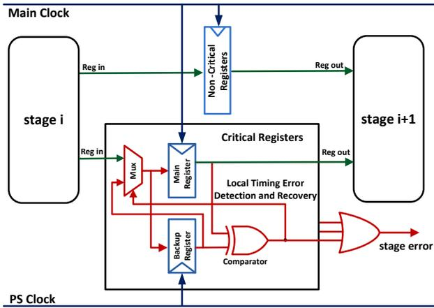
Fig. 1. Typical pipeline stage in a Reliably Overclocked Processor. Local timing error detection and recovery scheme for critical registers is shown in detail.
