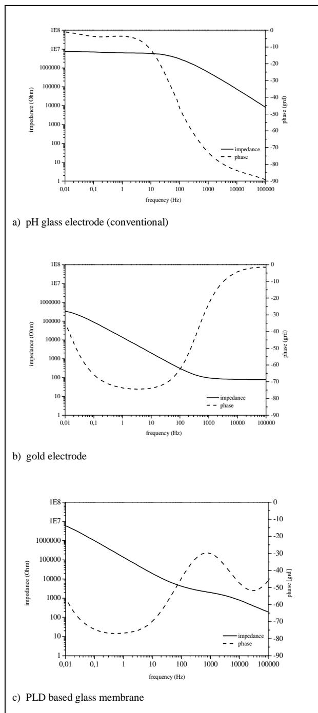
Figure 17. Impedance spectra in a NBS-buffer solution (pH=6.86)
