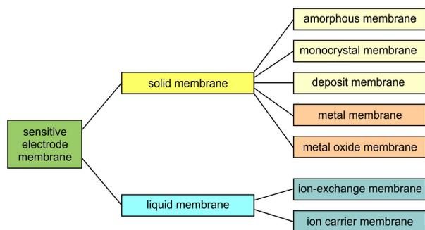
Figure 1. Classification of membrane materials for electrochemical sensors
