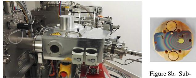
Figure 8a. Transfer device with mask and substrate handler
