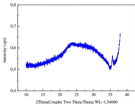
Figure 16. Diffractogram of pH glass thin film
