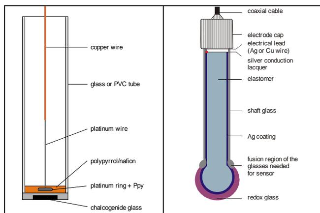
Figure 3. Schematic drawing of a chalcogenide glass electrode [8]
