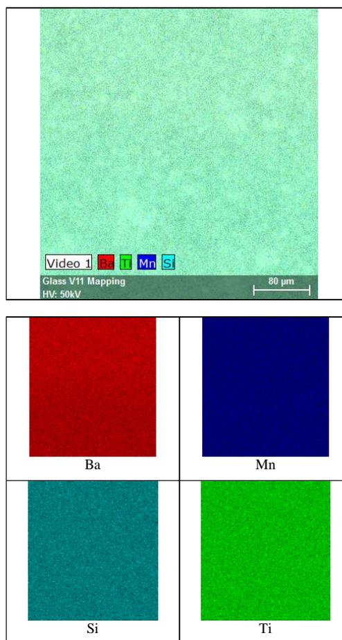
Figure 10. Element mapping of a PLD-based pH glass thin film
