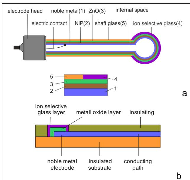
Figure 5. All solid state pH glass electrodes based on ZnO as interlayer
