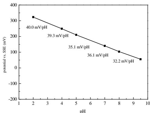
Figure 18. Potential measurement with thin-film pH glass electrode in TSC-buffer solutions
