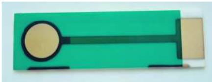
Figure 11: pH thin film electrode
