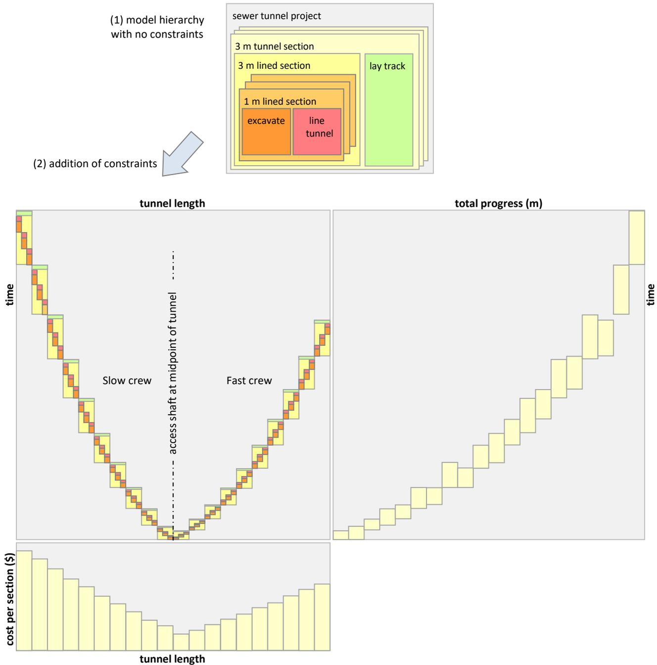
Figure 4. Foresight model of a sewer tunneling operation.
