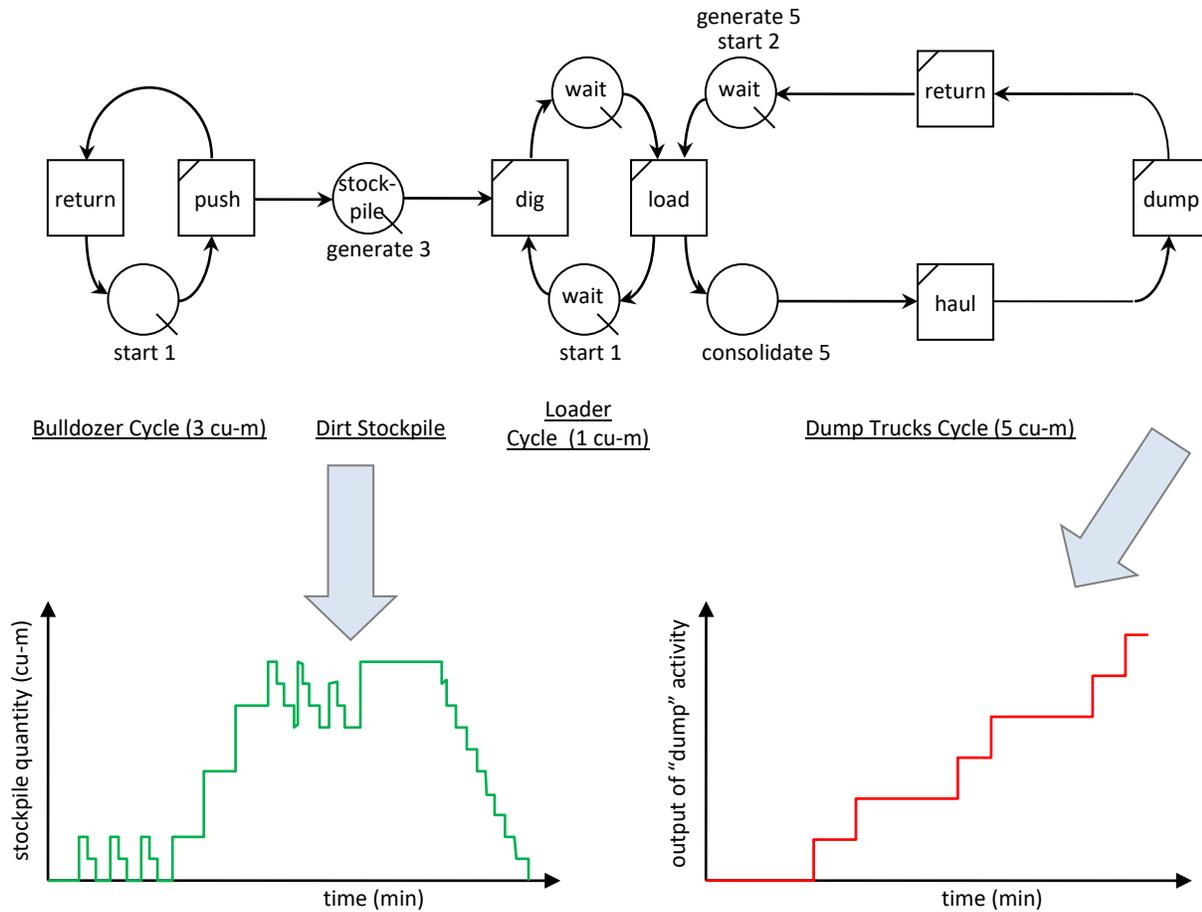
Figure 2. CYCLONE simulation model of an earthmoving operation.
