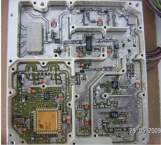
Figure 2. Uncovered on-board transceiver EM
