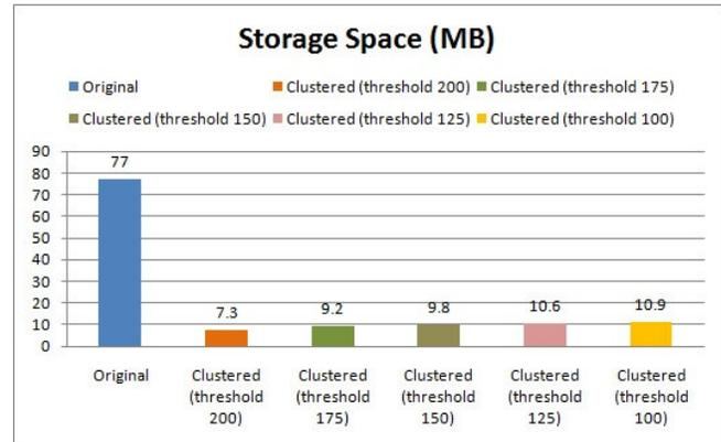
Figure 11. Storage space requirements for different thresholds.
