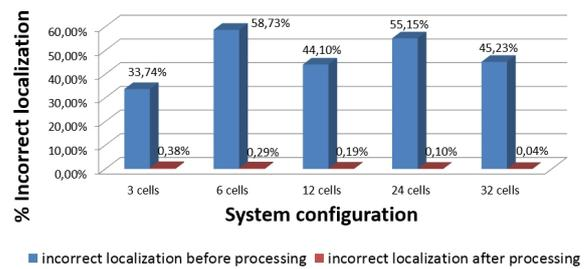
Figure 5. Percentage of incorrect localizations before and after the RCP algorithm processing for different RFID system configurations.
