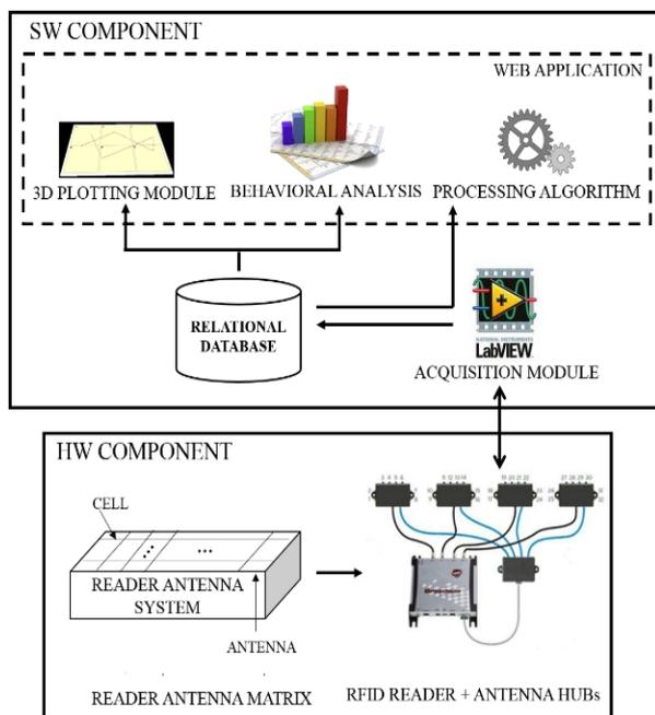
Figure 1. System architecture.
