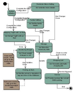
Figure 3. State Transition diagram of Smart Kitchen Cabinet
