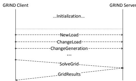
Fig. 3. An example of a message flow following the GRIND protocol
