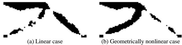
Figure 4. Optimal topology using  $MPE$
