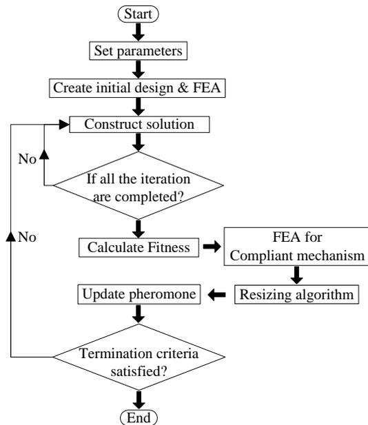
Figure 2. Flowchart of the MACO for compliant mechanisms
