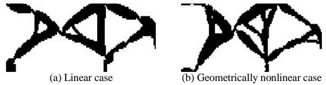
Figure 9. Optimal topology using  $wMPE+(1-w)SE$  ( $w = 0.8$ )
