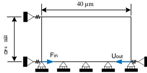
Figure 3. Design domain of a force inverter
