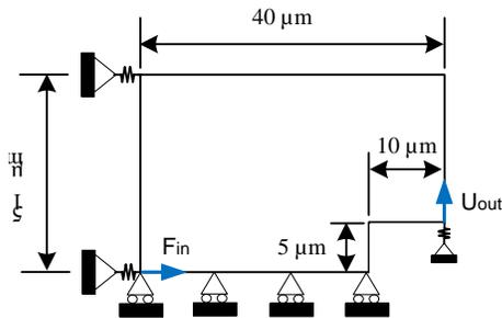
Figure 7. Design domain of a gripper mechanism
