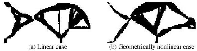
Figure 10. Optimal topology using  $MPE/SE$
