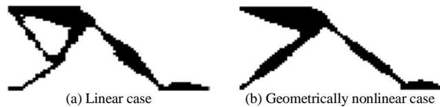
Figure 6. Optimal topology using  $MPE/SE$
