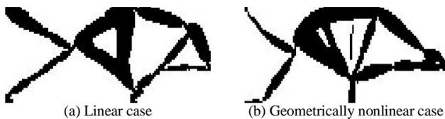
Figure 8. Optimal topology using  $MPE$
