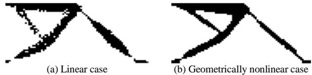
Figure 5. Optimal topology using  $wMPE+(1-w)SE$  ( $w = 0.8$ )
