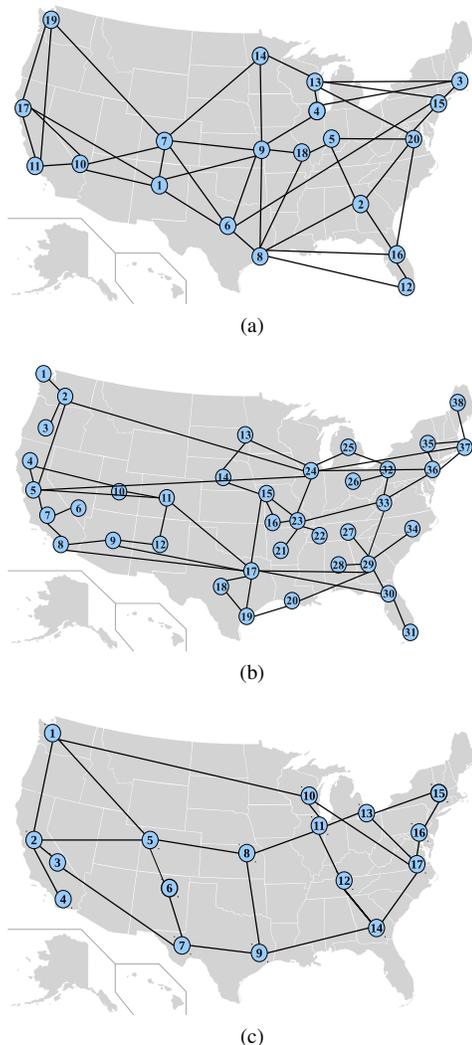
Figure 1: (a) Sample DCS composed of 20 nodes. (b) DCS interconnected by means of the AT&T IP backbone network 2Q2000 [27]. (c) DCS interconnected by means of a simplified version of the AT&T IP backbone network 2Q2000 [27].
