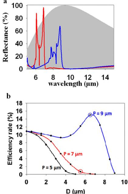
Figure 3. a) Reflection spectra for:  $P = 7 \mu\text{m}$  and  $D = 5.5 \mu\text{m}$  (red curve) and  $P = 9 \mu\text{m}$  and  $D = 6.5 \mu\text{m}$  (blue curve) with  $h = 4 \mu\text{m}$  b) Evolution of the efficient rate  $\eta$  as a function of  $D$ , for three periods  $P$  ( $h = 4 \mu\text{m}$ ). The circled dots correspond to the position of the two reflection spectra in a).
