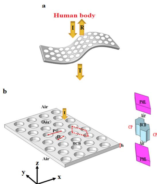
Figure 1. a) Principal scheme of the system with the direction of the incident (I), reflective (R) and transmissive (T) electromagnetic waves. b) (left) 3D view of the BCB membrane where  $h$  is the thickness,  $D$  the diameter and  $P$  the period. (Right) Elementary unit cell used for the FEM calculation with the absorbing (PML) and periodic (CP) boundary conditions.
