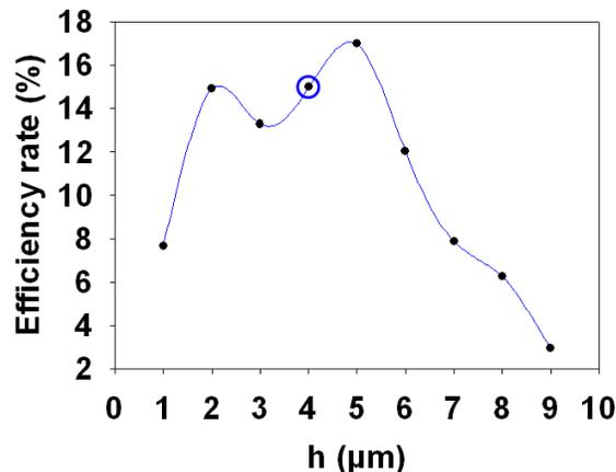
Figure 4. Evolution of the efficiency reflection coefficient  $\eta$  as a function of  $h$ , with  $P = 9 \mu\text{m}$  and  $D = 6.5 \mu\text{m}$ . The circled dot corresponds to the position of the blue reflection spectrum in a).
