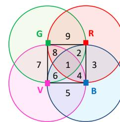
Figure 2. Unit cell (LED array = RGBV color spots).
