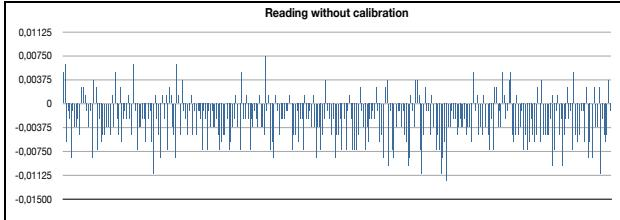
Figure 3. Acquired values from gyroscope without calibration (1,000 readings)
