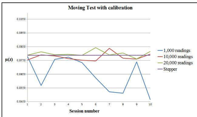
Figure 6. Gyroscope's average angular velocity for 1,000, 10,000 and 20,000 readings compared to the reference angular velocity of the Stepper Motor with calibration
