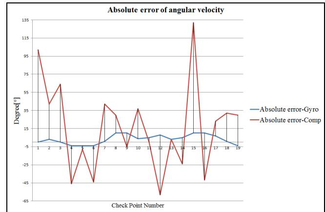
Figure 8. Comparison between the absolute error of Gyroscope and Compass for an indoor path made of 19 CheckPoints
