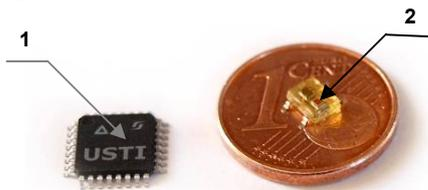
Figure 1. USTI (1), and light-to-digital converter S9705 (2).
