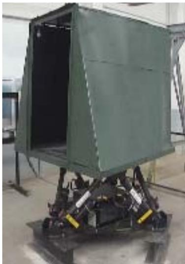
Fig. 5: The MOOG 6DOF 2000E 170 E131 motion platform.
