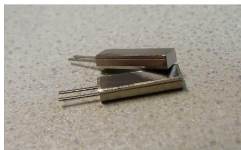
Figure 6. Custom Kovar housing 1.9 x 3.1 x 10.0 mm 3 .
