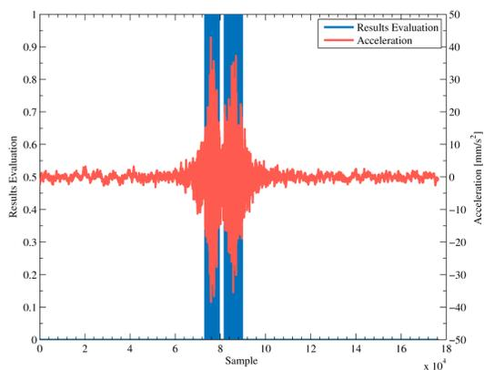
Fig. 5. Recognition with the filter of a passing car with 50 km/h in 30 cm distance.
