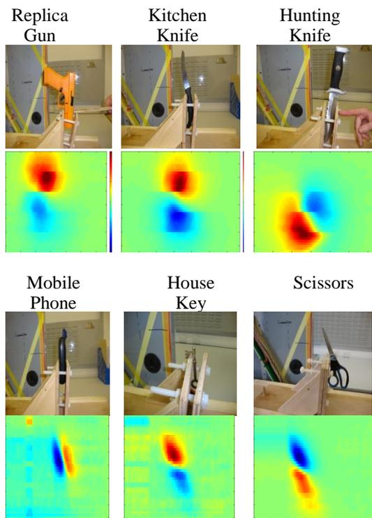
Fig. 5: Samples with the equivalent EMIs.
