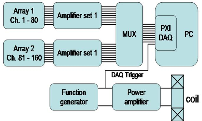
Fig. 3: System block diagram
