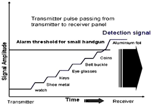
Fig. 2: Cumulative signal effects in active walkthrough weapon detector.
