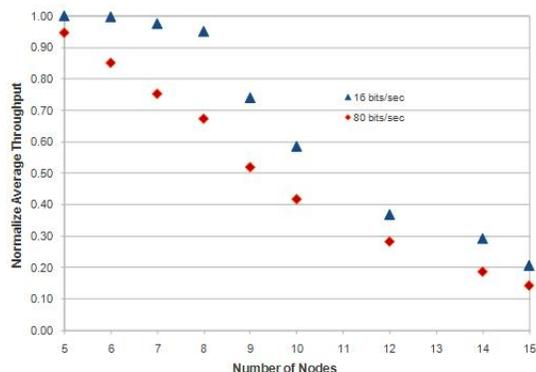
Figure 6. Average node throughput for one-hop cluster networks where nodes send data at 16 bits/second and 80 bits/second respectively normalized by that packet generation rate.
