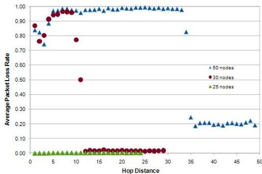
Figure 8. Average Packet Loss as a function of hop-distance to the fusion node for linear networks of length 25, 30, 50 nodes. Data packets are generated at each node at a rate of 80 bits/sec.
