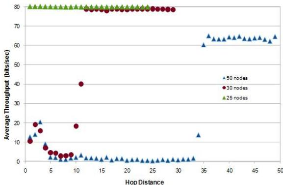
Figure 9. Average Throughput as a function of hop-distance to the fusion node for linear networks of length 25, 30, 50 nodes. Data packets are generated at each node at a rate of 80 bits/sec.
