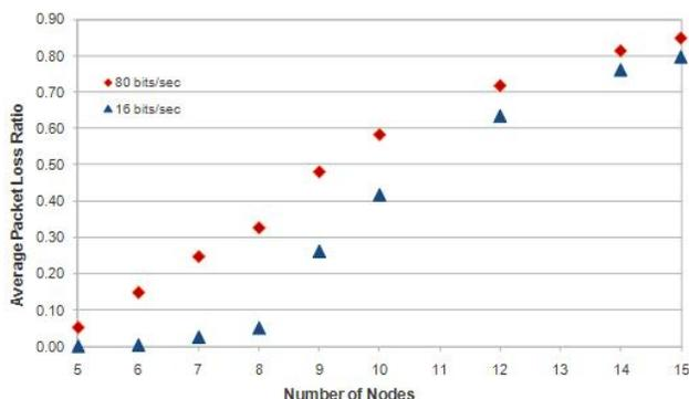
Figure 5. Average Packet Loss Ratio for one-hop cluster networks where sensor nodes send data at 16bits/sec and 80bits/sec respectively.
