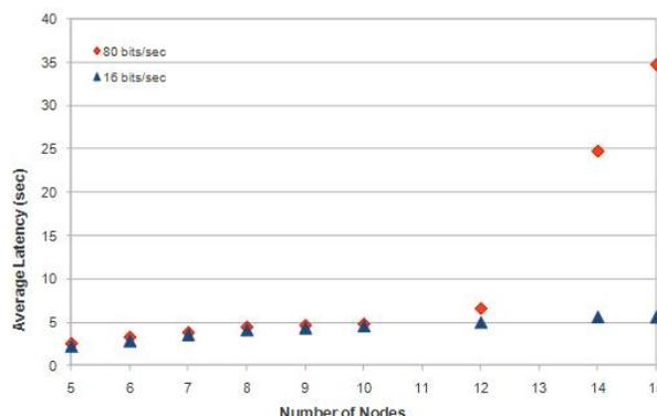
Figure 4. Average Latency for one-hop cluster networks where each sensor node sends data at 16bits/sec and 80bits/sec respectively.
