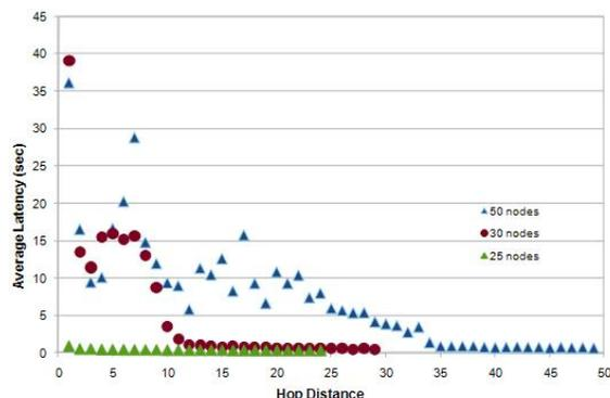
Figure 7. The Average Latency for a multi-hop linear network plotted as a function of hop distance to the fusion node for linear networks of length 25, 30, 50 nodes. Data packets are generated at each node at a rate of 80 bits/sec.
