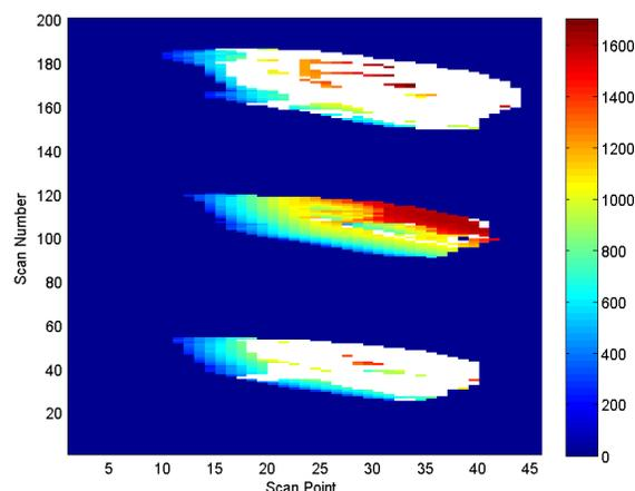
Figure 4: Representation of three cars (height)
