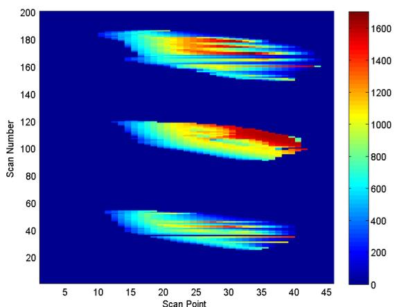
Figure 5: Representation of three cars (interpolated)
