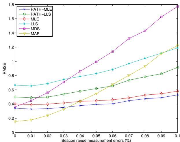
Fig. 3. RMSEs of location estimates via  $\kappa$ : rectangular grid network.
