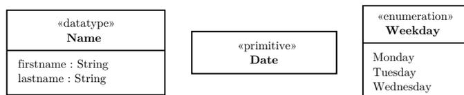
Fig. 1. Examples for datatypes in UML. Left: user-defined datatype with two components. Center: user-defined primitive datatype. Right: Enumeration with three allowed values.
