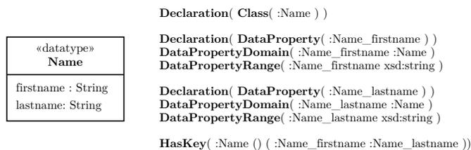
Fig. 5. Example for the transformation of a complex datatype.
