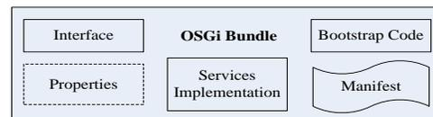
Figure 10. Structure of an OSGi bundle providing properties
