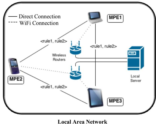
Figure 4. A possible network of distributed MPEs
