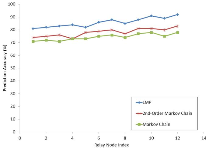
Fig. 5. Comparison of prediction accuracy for the proposed LMP algorithm, generic Markov chain and second-order Markov chain for User Node 1 in networks with 120 users, 14 relay nodes and 1 base station
