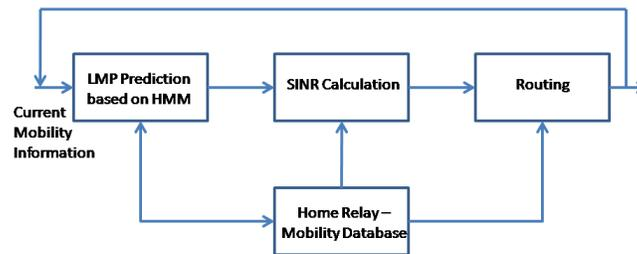
Fig. 2. Block diagram that illustrates the interaction between the LMP algorithm and the interference aware routing algorithm. The home relay runs the prediction algorithm and the SINR calculation for the routing procedure
