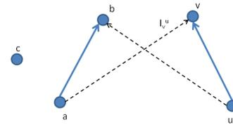
(a) Node  $a$  is transmitting to node  $b$  and node  $u$  is transmitting to node  $v$
