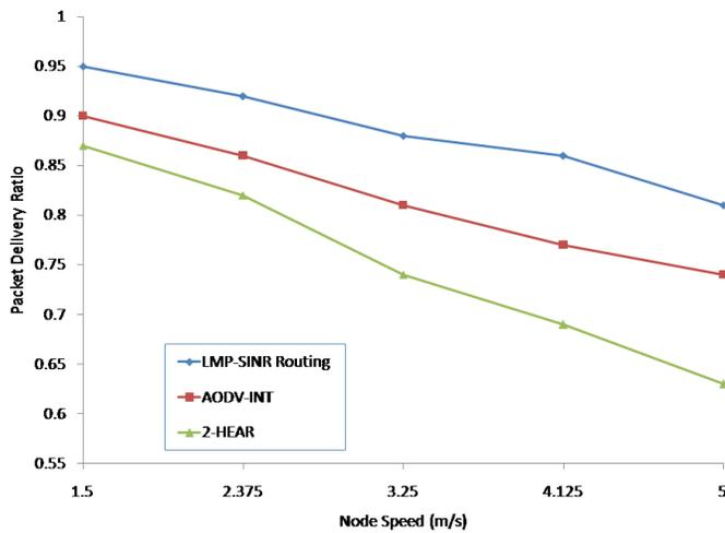
Fig. 8. Packet delivery ratio versus varying node speeds for  $T = 1ms$
